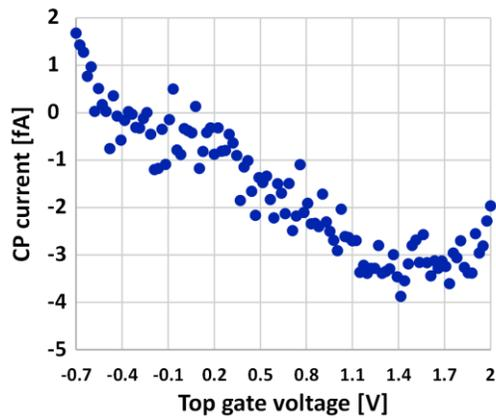
Figure 6 CP current when there is no defect at the interface of the MOSFET. The change in CP current is the baseline drift of the current amplifier.
