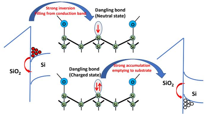
Figure 2, Illustration of how the Pauli’s exclusion principle limits the dangling bond interface defect to accommodate a maximum of two electrons. Since it contains one electron, it can only accept one additional electron with opposite spin. During the inversion half cycle, this additional electron is provided by the inversion layer. During the accumulation cycle, one of the electron is emitted to the substrate thereby completes one charge transfer.
