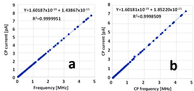
Figure 5 CP current as a function of frequency is a linear function with a slope equals Coulombs. **a** and **b** are two examples with **b** has a slightly higher noise level and therefore a poorer fit.
