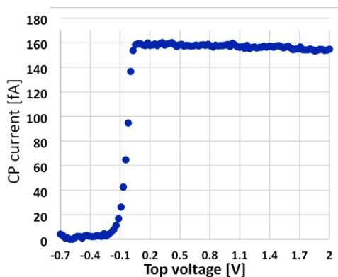
Figure 4 The CP current from a single interface defect. A single step-rise to 0.16 pA level (1 defect) is observed.
