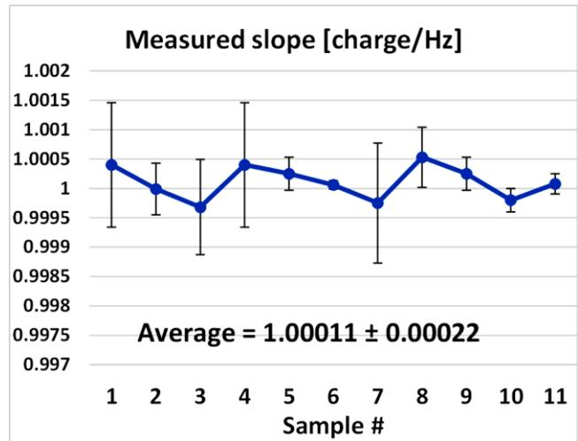
Figure 7 The measured CP vs frequency slope after converting Coulomb to electron charge for 11 single defect devices. The average of all 11 devices is also shown. The errors bars represent standard deviation.
