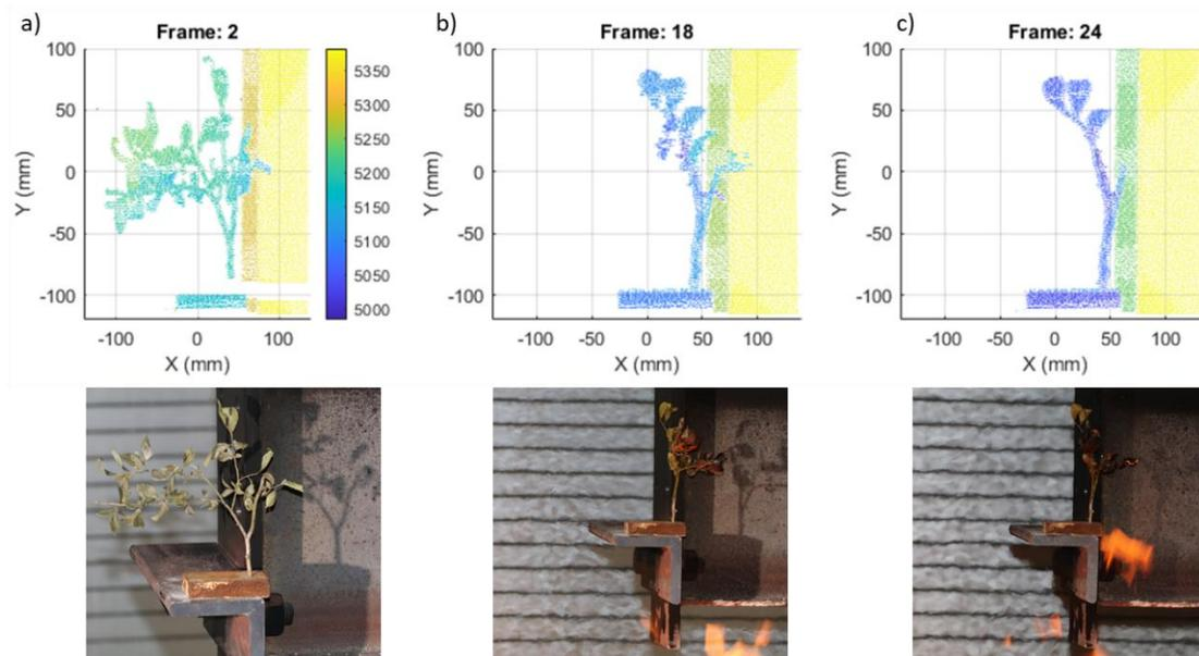
Fig. 3. Point clouds and photographs of a blueberry bush branch heated over a 100 kW fire (false color for range). a) 66 s after fire ignition. b) 600 s after fire ignition. b) 800 s after fire ignition.
