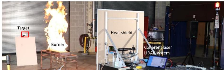
Fig. 1. Experimental setup. Target objects are placed either behind or in the flames produced by a natural gas burner. The FireLiDAR is protected by a heat shield with a quartz glass window. The laser light around 1550 nm from an FMCW LiDAR is coupled into free-space with a beam expander and is scanned across an object with a steering mirror.
