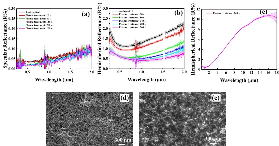
**Figure 1:** (a) Specular and (b) hemispherical reflectance of as-deposited and plasma-treated sample ( $0.25\ \mu\text{m} - 2\ \mu\text{m}$ ), (c) hemispherical reflectance in  $0.25\ \mu\text{m} - 18\ \mu\text{m}$  range after 260 s of  $\text{O}_2$  plasma treatment. Uncertainty is shown by shading; Surface morphology of (d) as-deposited and (e) 260 s plasma-treated sample.
