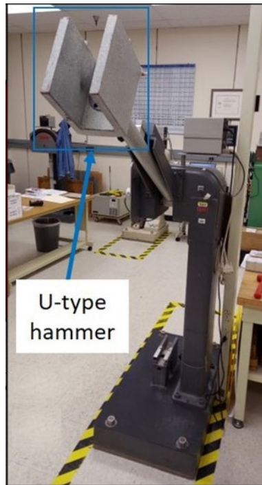
Fig. 1. Reference Charpy machine (U-type hammer) used for the 1 st series of tests performed at NIST on lots LL-189 and HH-190.
