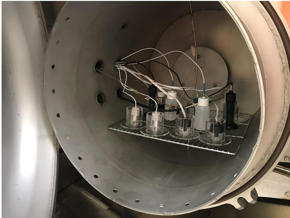
**Fig. 2.** DDL installation during environmental calibration.
