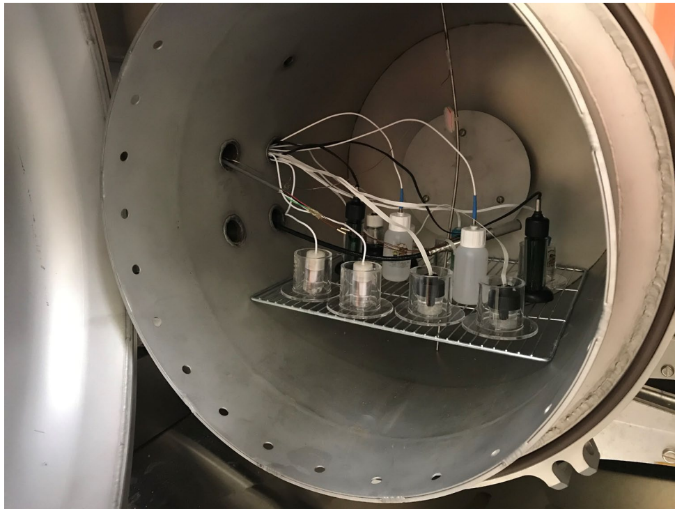
Fig. 2. DDL installation during environmental calibration.
