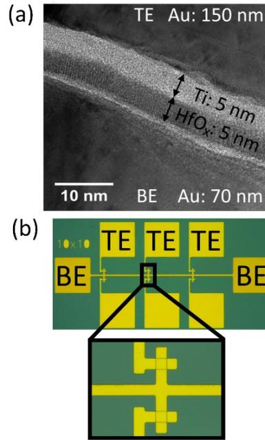
**Figure 1.** (a) Cross-sectional TEM image of an as-deposited device stack. This confirms the deposition of a  $\approx 5$  nm titanium capping layer and  $\approx 5$  nm HfO<sub>x</sub> active area. (b) Device structure used to create RRAM crossbars. This design ensures no electrical sneak paths are possible due to the electrical isolation of each device.
