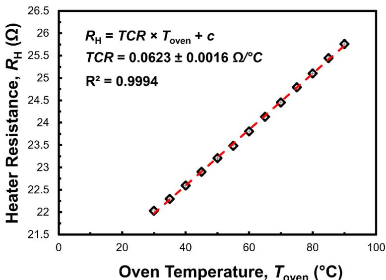
**Figure S10.** Measured resistance (4-point configuration) of a  $\approx 200$  nm thick gold microheater as a function of the oven temperature. A linear fit using a Monte Carlo method was used to extract
