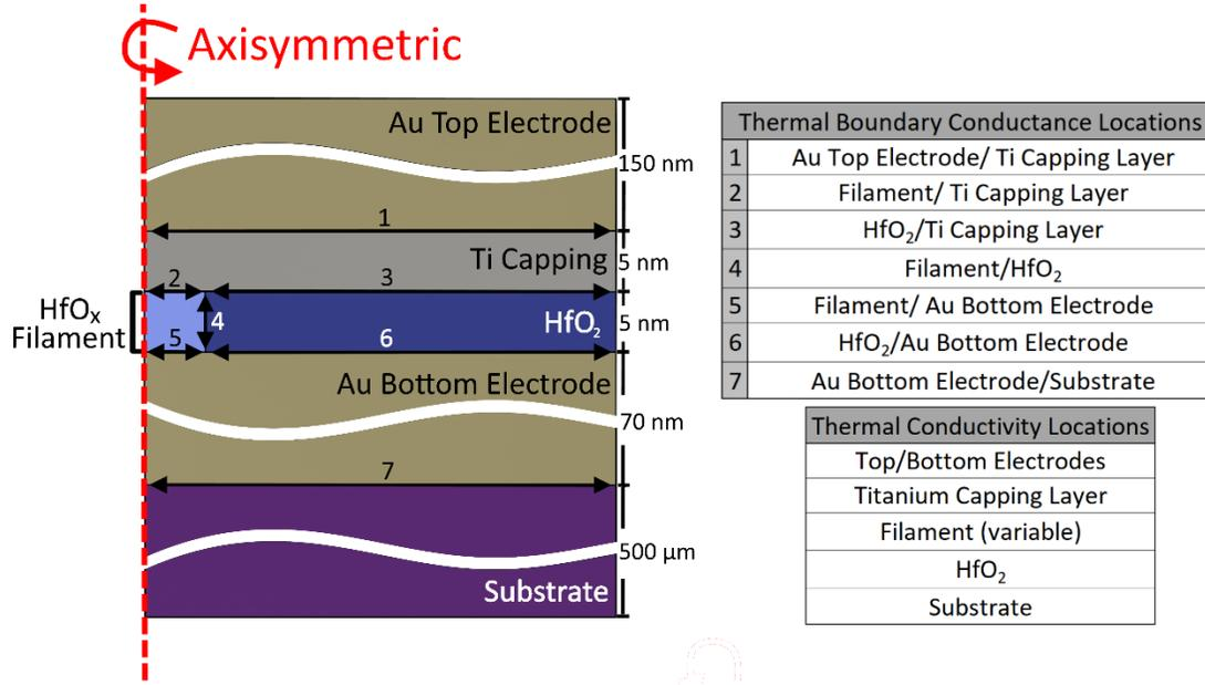
**Figure 7.** Simulated model geometry annotated with thermal conductivity and boundary locations varied in the parametric studies. The thermal conductivity of the filament is variable with the concentration of oxygen vacancies and is not changed in any of the parametric studies (Equation S1). Each of these thermal conductivities and interfacial thermal conductances is changed independently while all other parameters are constant according to Table S2.
