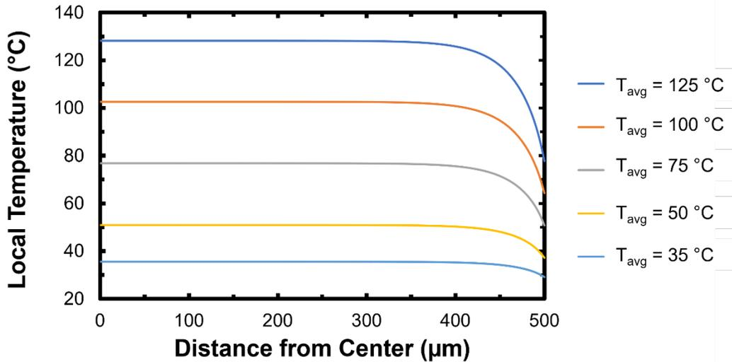
**Figure S11.** Spatial temperature profiles extracted from the thermal Finite Element Model (FEM) used to simulate Joule heating in the gold microheater. The heating was modelled for five different average temperatures ( $T_{avg}$ ) corresponding to the conditions used for calibrating the SThM tips.
