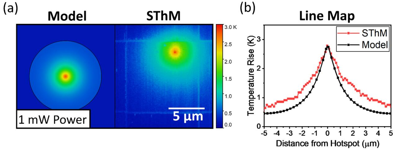
**Figure 3.** (a) Maps of the top electrode temperature obtained with the multiphysics model (left) and SThM (right) showing good agreement when a constant 1 mW of power goes through the filament. (b) Top electrode temperature profile passing through center of the hot spot for simulation and SThM.
