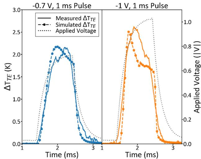
**Figure 5.** Comparison between the  $\Delta T_{\text{TE}}$  measured in the experiment on top of the filament and the  $\Delta T_{\text{TE}}$  obtained by the model during voltage pulsing under identical conditions (-0.7 V, left and
