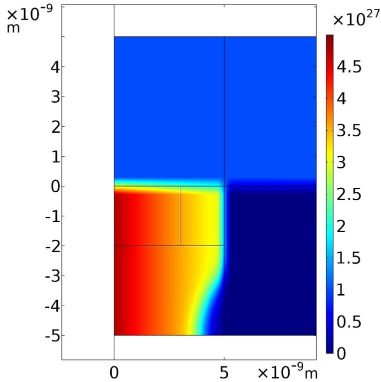
**Figure S12.** Initial vacancy distribution for the device in the low resistance state. The model is unable to simulate the forming process. A shape with a smaller diameter near the bottom electrode is assumed. This filament has proven to match the electrical and thermal behavior of our devices well.
