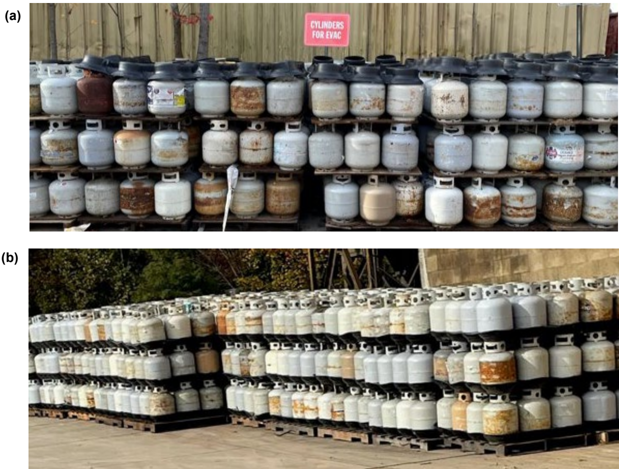
Fig. 5. (a) Used nominal 20 lb cylinders to be evacuated (“EVAC”) and (b) cylinders following EVAC in preparation for a point of pack tare weight (TW) assessment.
