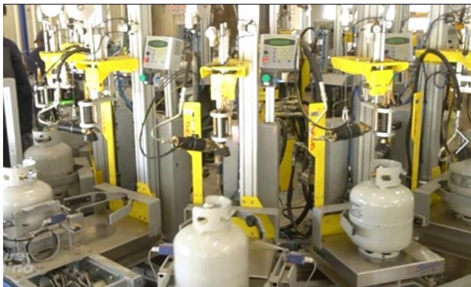
Fig. 12. A typical manufacturing facility automatic filling process of nominal 20 lb cylinders with propane by weight.
