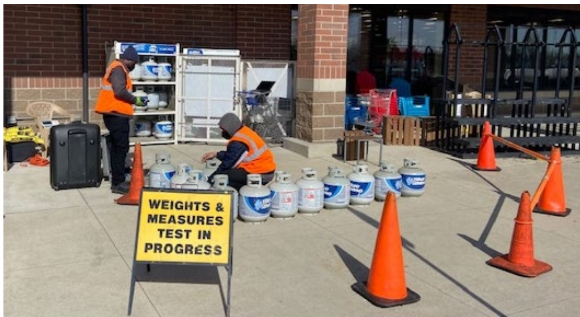
Fig. 4. An example of a weights and measures net weight compliance inspection at an exchange location. (Credit: Lucas County, OH and used with permission)
