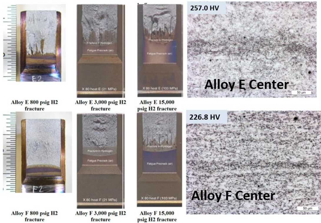
FIGURE 8. Surface separations from E1820 fracture toughness tests in hydrogen of two X80 steels from the 2000s where the top one contains molybdenum and the bottom one does not
