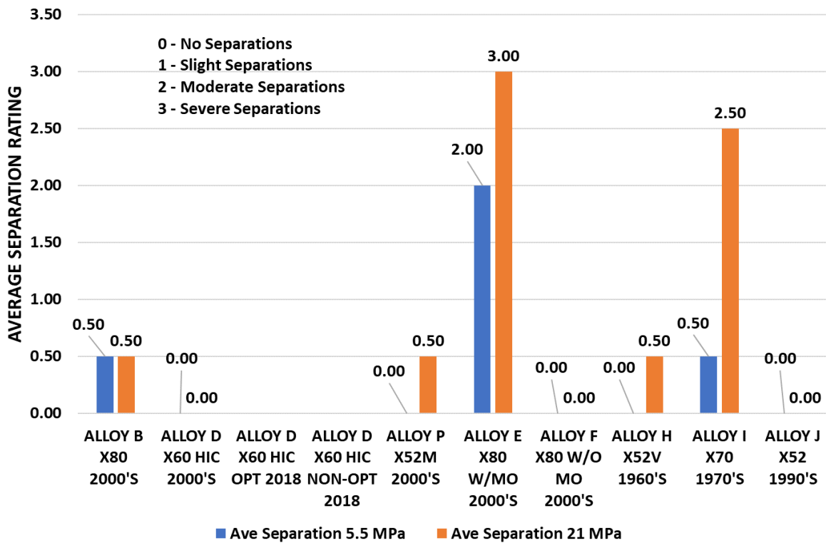
FIGURE 6. Rankings of CT specimen fracture surface separations from E1820 fracture toughness tests in hydrogen
