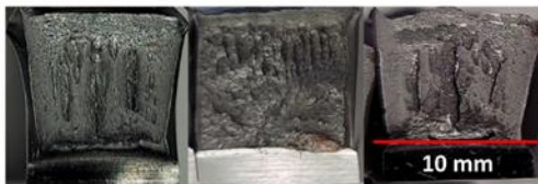
Air TCVN Ranking 3 - Severe Visual Separations
