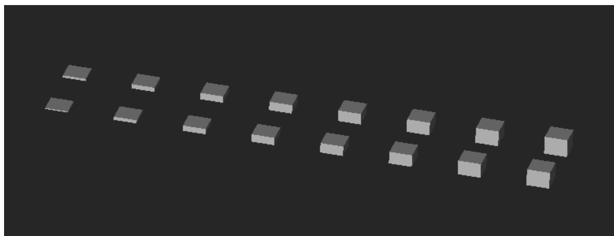
Figure S2. CAD model used for projection of the working curve. Each block measures 1x1 mm 2 at the base.
