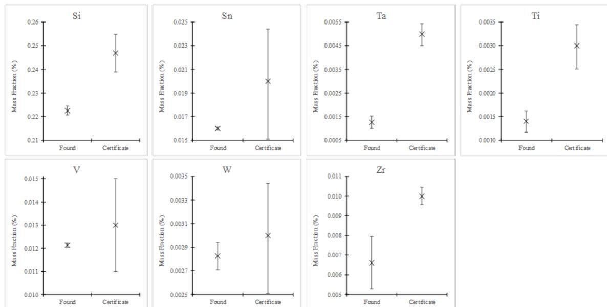
**Fig. 5.** Graphical comparisons of found results for SRM 1270 from NIST WDXRF to certificate values for SRM 1270. Error bars for found results are the expanded uncertainty estimates,  $U_{k=2}$ , from **Table 27a** and **b**. Error bars for certified elements Si and V are  $2u$  from **Table 27b**, where  $u$  is the standard uncertainty estimate from the certificate. Error bars for information values for Sn, Ta, Ti, W, and Zr assume the values were rounded from more precise results.
