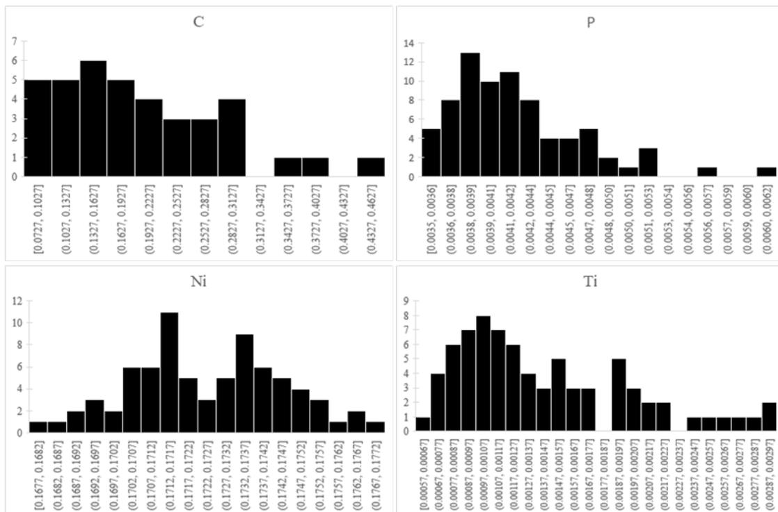
**Fig. 3.** Histograms of measured results by WDXRF for elements in SRM 1270a showing skewed distributions for C, P, and Ti and a bimodal distribution for Ni. Values on the horizontal axes are mass fractions in percent (%). Values on the vertical axes are the counts of results in each bin of the histogram.
