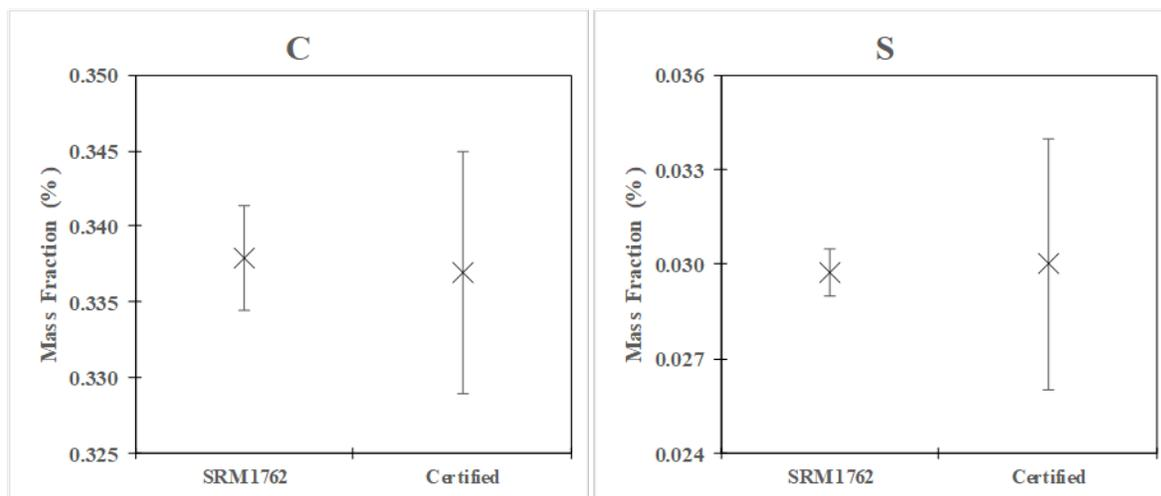
**Fig. 7.** Graphical comparison of collaborator CID results for total carbon and sulfur in SRM 1762 to the certified values for SRM 1762. Error bars for test results are two times the repeatability standard deviation for the measured results. For the certified values, they are two times the combined standard uncertainty of the certified value.
