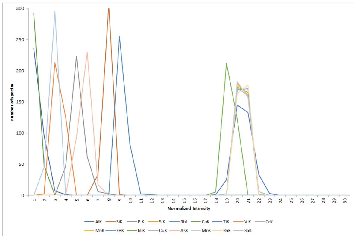
**Fig. 2.** Distributions of measured count rates across a single disk of SRM 1270a with measurements made using a 1 mm diameter X-ray beam and measured locations spaced 1 mm apart in a 17 x 20 grid. Measured lines RhL and RhK are characteristic lines from the Rh X-ray tube anode scattered from the steel sample surface. Rhodium is not present in the steel sample.
