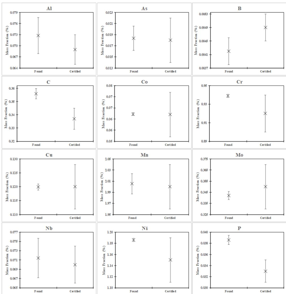
**Fig. 6a.** Comparisons of collaborator found results for SRM 1762. Error bars for found results are two times the repeatability standard deviation,  $2s$ . Error bars for certified values are two times the combined standard uncertainty estimate,  $2u$ .
