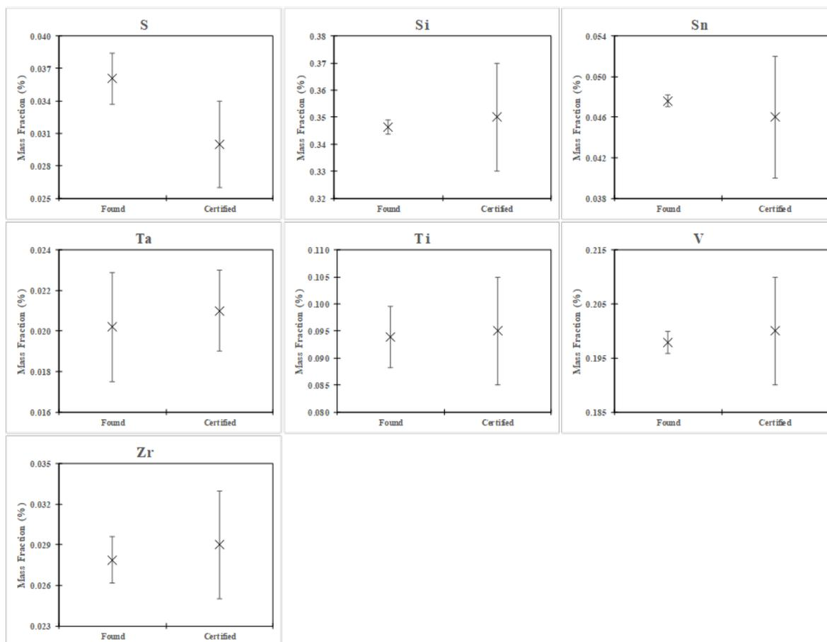
**Fig. 6b.** Comparisons of collaborator found results for SRM 1762. Error bars for found results are two times the repeatability standard deviation,  $2s$ . Error bars for certified values are two times the combined standard uncertainty estimate,  $2u$ .
