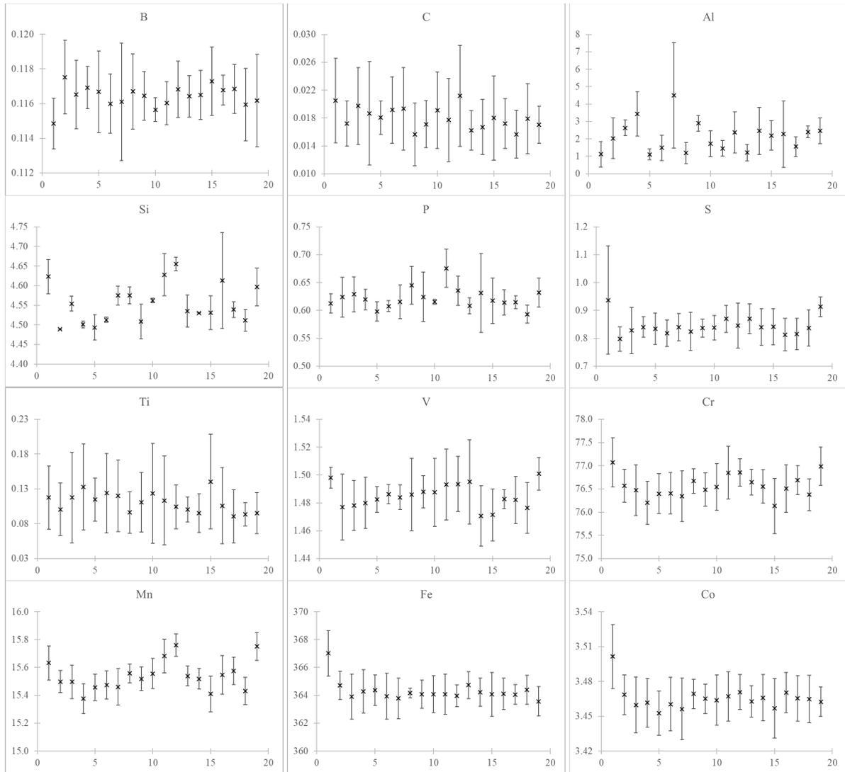
**Fig. 1a.** Distributions of elements among the disks of SRM 1270a Low Alloy Steel. All error bars are the standard deviation of  $n = 4$  individual measurements ( $n = 2$  for Al, Si, Zr) for the disk. Values on the horizontal axes are the specimen disks numbered from 1 to 19 in order from top to bottom as shown in the Analysis of Variance tables in section 3.5. Values on the vertical axes are X-ray signal intensity in thousands of counts per second (kCPS).
