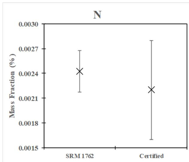
**Fig. 8.** Graphical comparison of collaborator IGF results for total nitrogen in SRM 1762 to the certified value for SRM 1762. Error bars for test results are two times the repeatability standard deviation for the measured results. For the certified value, they are two times the combined standard uncertainty of the certified value.
