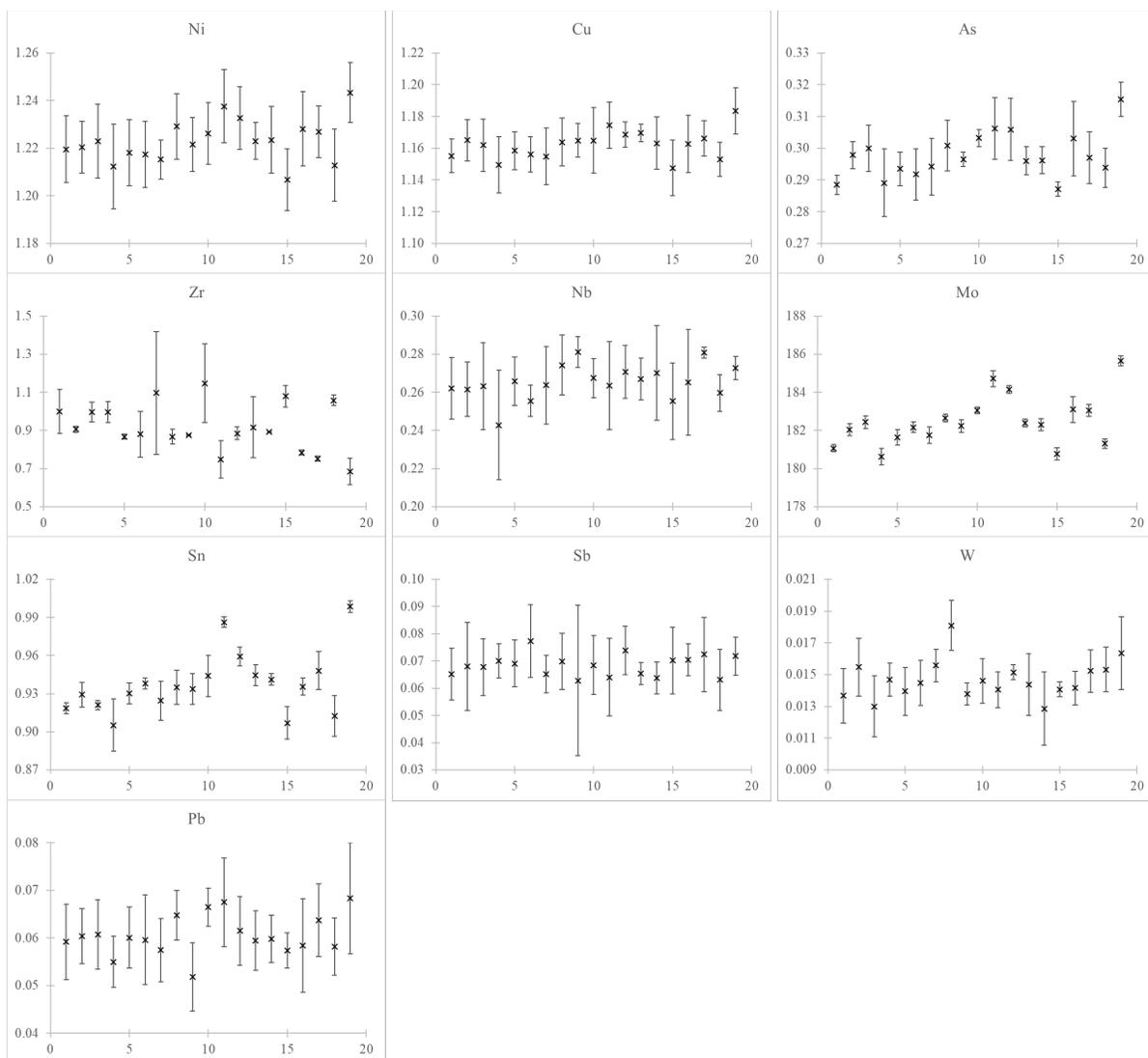
**Fig. 1b.** Distributions of elements among the disks of SRM 1270a Low Alloy Steel. All error bars are the standard deviation of  $n = 4$  individual measurements ( $n = 2$  for Al, Si, Zr) for the disk. Values on the horizontal axes are the specimen disks numbered from 1 to 19 in order from top to bottom as shown in the Analysis of Variance tables in section 3.5. Values on the vertical axes are X-ray signal intensity in thousands of counts per second (kCPS).
