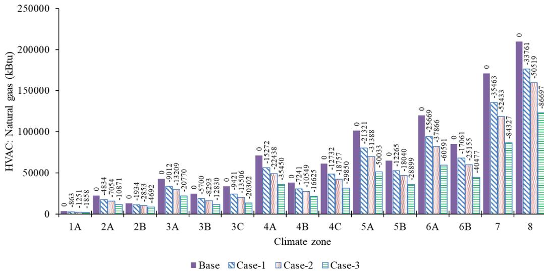
Figure 2 Natural gas consumption and savings for HVAC-related gas use at four levels of air leakage compared to the base case
