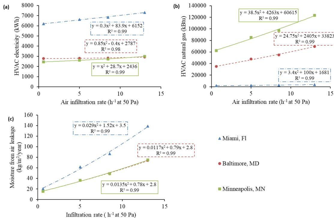
Figure 4 Quadratic regression with infiltration rate as dependent variable (a) HVAC electricity consumption (b) HVAC natural gas consumption (c) Moisture transfer from air leakage
