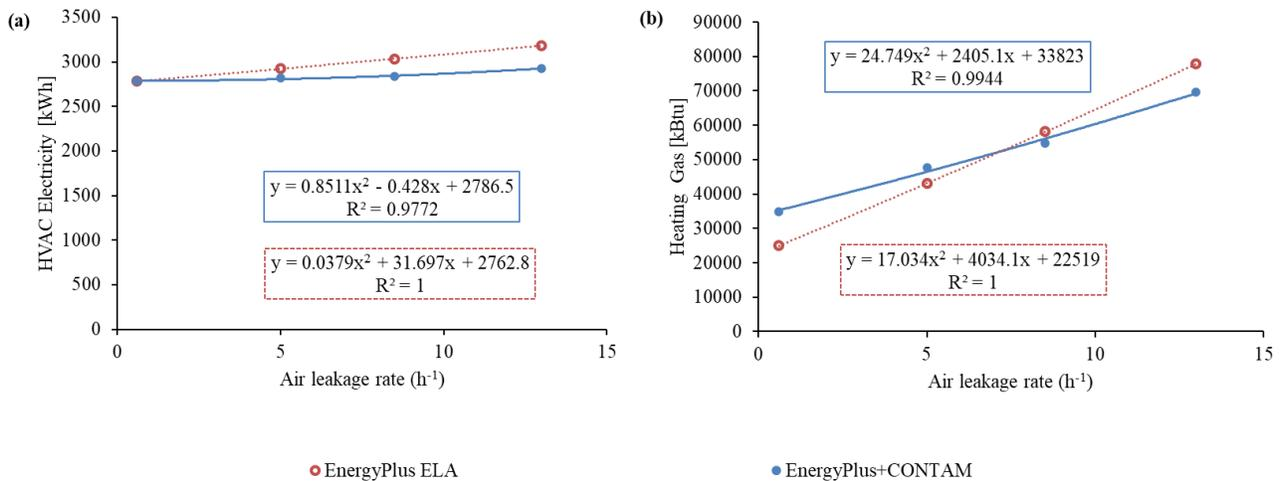
Figure 5 Comparison between energy consumption using EnergyPlus ELA and EnergyPlus+CONTAM approaches for incorporating infiltration at different air leakage rates in Baltimore, MD
