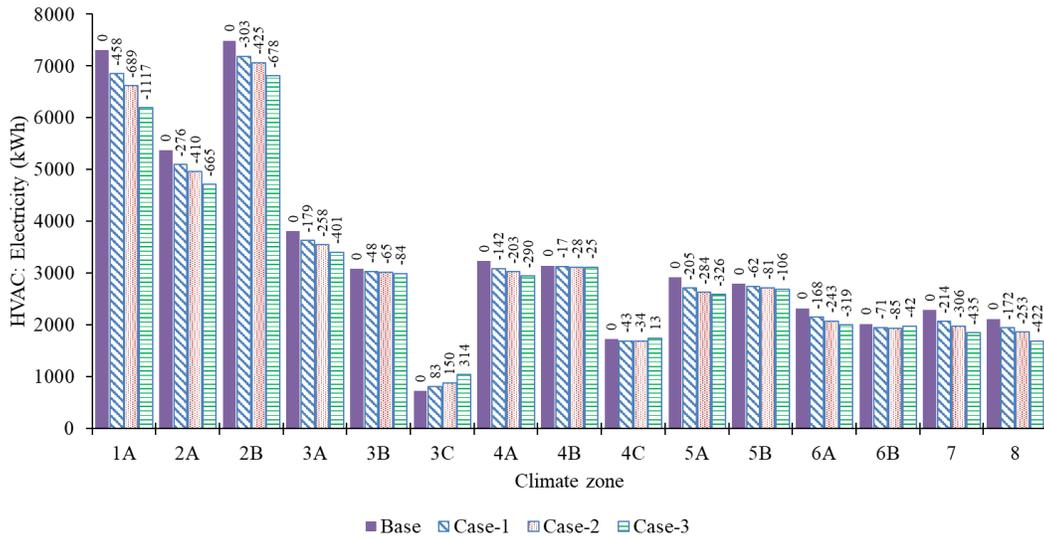
Figure 1 Electricity consumption and savings for HVAC-related electricity use at four levels of air leakage compared to the base case
