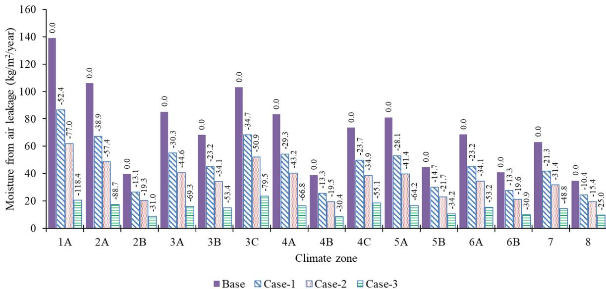
Figure 3 Moisture transfer per unit envelope area from infiltration at four levels of air leakage and reduction in moisture transfer compared to the base case
