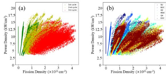
Fig. 4. A distribution of the correlation between power and fission densities throughout the core at (a) multiple cycles and (b) multiple cycle states.
