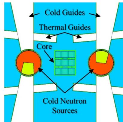
Fig. 2. A top view of the NNS core and cold neutron sources.
