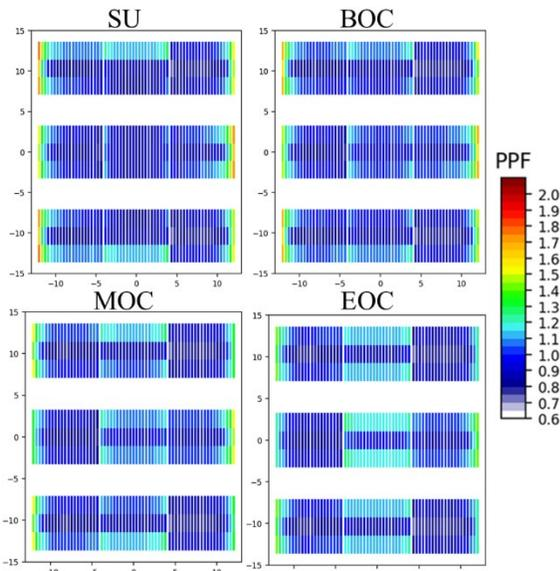
Fig. 3. A spatial distribution of the power peaking factors at each fuel plate throughout the core.
