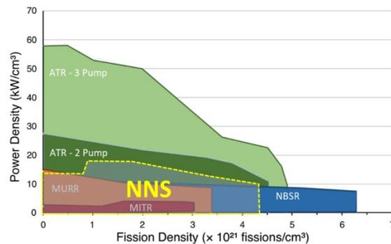
Fig. 5. The Power and fission density profile of the NNS compared to other high-performance research reactors (modified and reproduced from [7-8]).
