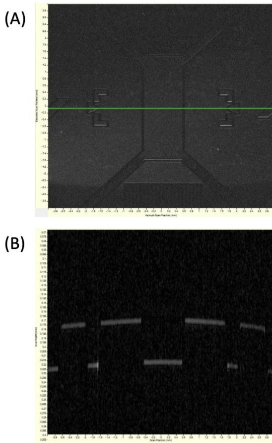
**Fig. 5.** (A) Volume intensity projection of the OCT image of the step height calibration standard. (B) The B-scan (depth) image corresponding to the green line slice drawn in (A).
