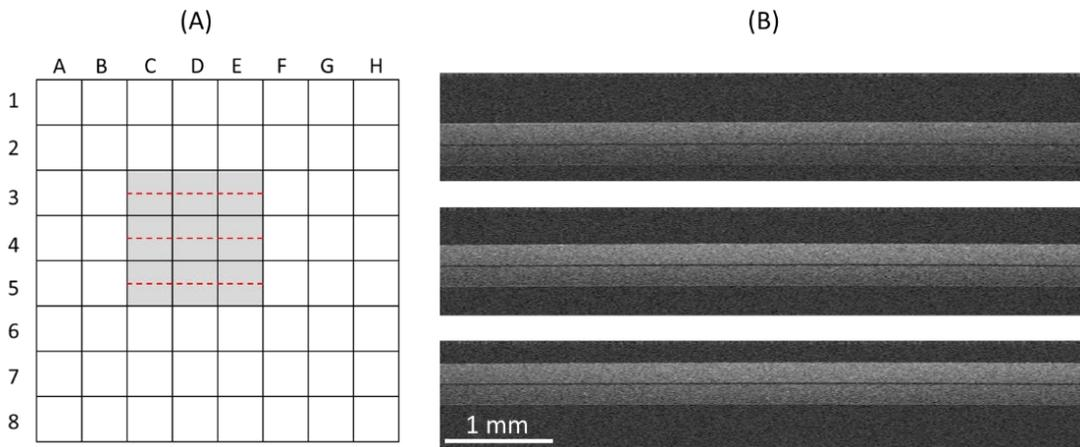
**Fig. 3.** Cross-section OCT images of the target regions of interest of a SRM. (A) Top view of a targeted imaging area (6 mm x 6 mm) of a SRM slide. (B) 3 B-scan (cross-section) images, 100<sup>th</sup> (upper), 300<sup>th</sup> (middle), and 500<sup>th</sup> (lower) of the 600 B-scans of the SRM 002, corresponding to the dotted red lines in (A). Although the images are acquired in pixels, a scale bar is shown which applies to the x-axis. The axial depth of the B-scan is approximately 1.1 mm.
