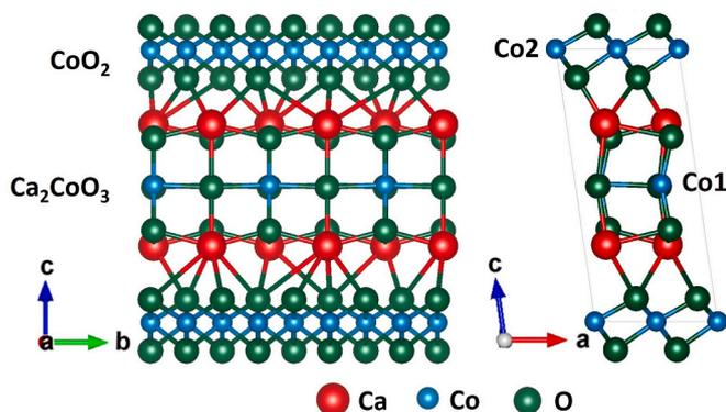
Fig. 2. The unit cell structure of  $\text{Ca}_3\text{Co}_4\text{O}_{9+\delta}$  showing the alternating subsystems of electrically conductive  $\text{CoO}_2$  sheets and insulating rock-salt-type  $\text{Ca}_2\text{CoO}_3$  layers.
