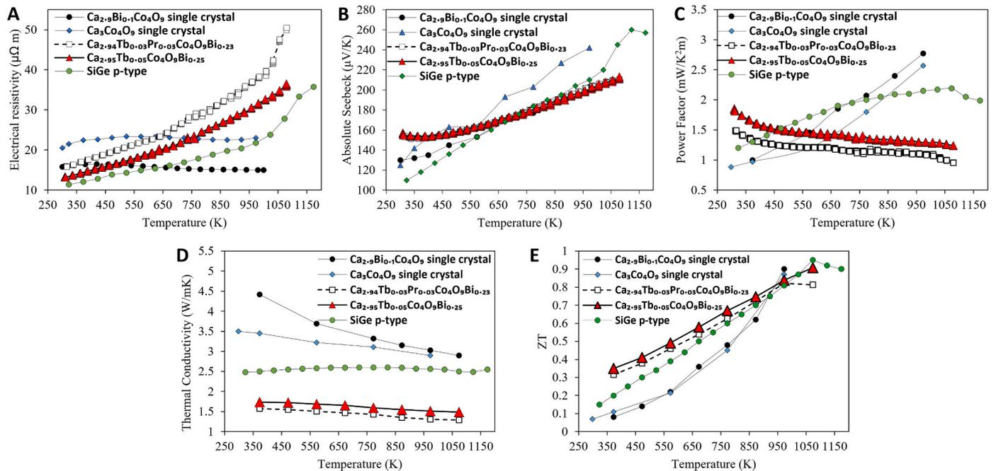
**Fig. 10.** Thermoelectric properties as function of temperature for several *p*-type materials [23,32,54]: (A)  $\rho$ , (B)  $S$ , (C)  $S^2\sigma$ , (D)  $\kappa$ , and (E)  $ZT$ . The current approach on grain boundary engineering successfully outperformed the  $ZT$  of single crystal  $\text{Ca}_3\text{Co}_4\text{O}_{9+\delta}$  and the conventional TE material SiGe. Reprinted (adapted) with permission from {Chem. Mater. 2020, 32, 22, 9730–9739}. Copyright {2020} American Chemical Society.
