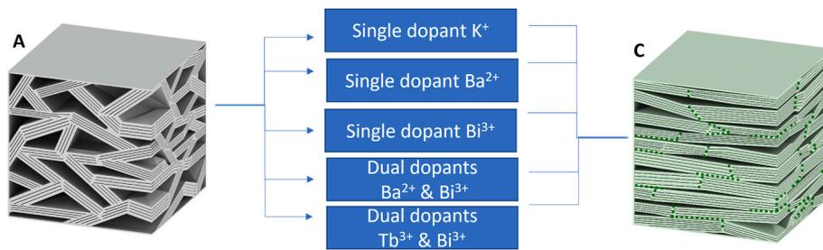
**Fig. 11.** Schematic showing the undoped (A)  $\text{Ca}_3\text{Co}_4\text{O}_{9+\delta}$  and (B) the single and dual element dopant approach to systematically tune the grain boundary and achieve the microstructure evolution. The improved alignment and crystal texture development is achieved with a variety of single and dual elements dopants. Reprinted (adapted) with permission from {Chem. Mater. 2020, 32, 22, 9730–9739}. Copyright {2020} American Chemical Society.
