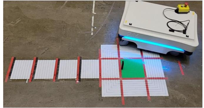
**FIGURE 11:** THE MOMENT WHEN THE A-UGV PASSES BY A SMALL OBSTACLE
