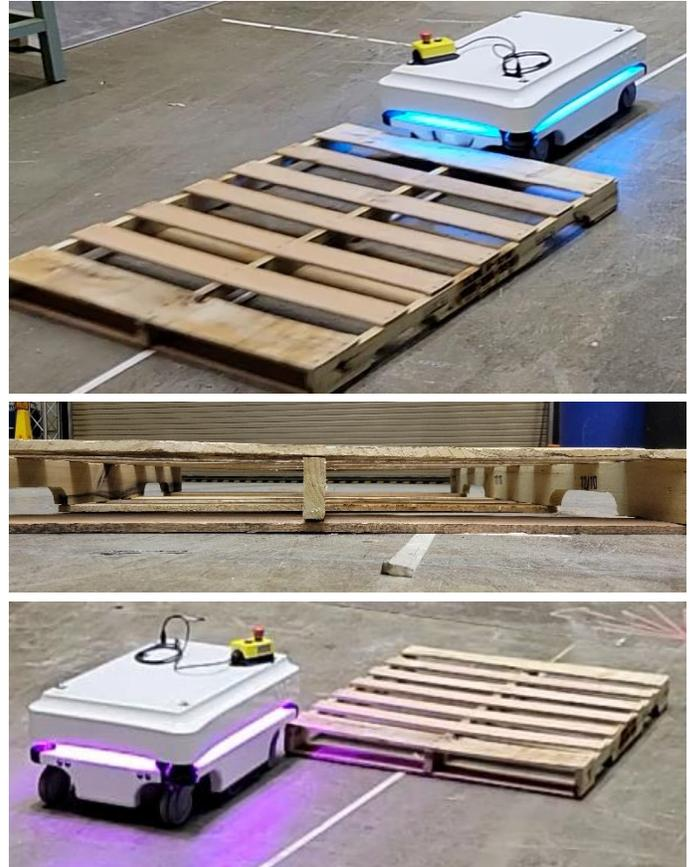
**FIGURE 1:** THE A-UGV COLLIDES WITH THE PALLET (TOP), THE PALLET IS ALIGNED IN A LESS DETECTABLE POSE (MIDDLE), AND THE PALLET BLOCKING A PORTION OF THE PATH (BOTTOM)
