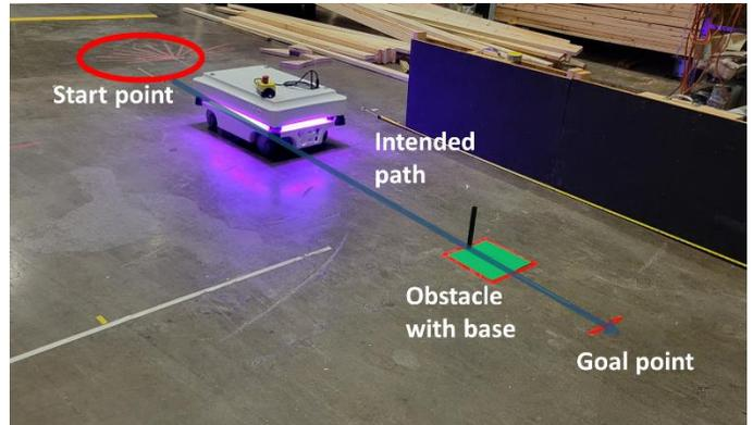
**FIGURE 7:** EXPERIMENT SETUP BEFORE A GRID INSTALLATION
