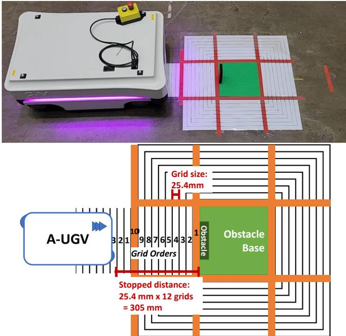
**FIGURE 9:** THE A-UGV STOPPED BETWEEN THE 12<sup>TH</sup> and 13<sup>TH</sup> MARKS(TOP), AND ITS PLANAR VIEW
