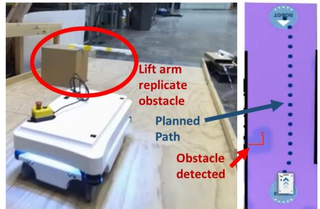
**FIGURE 5:** A PATH TO AVOID THE FORKLIFT ARM OBSTACLE
