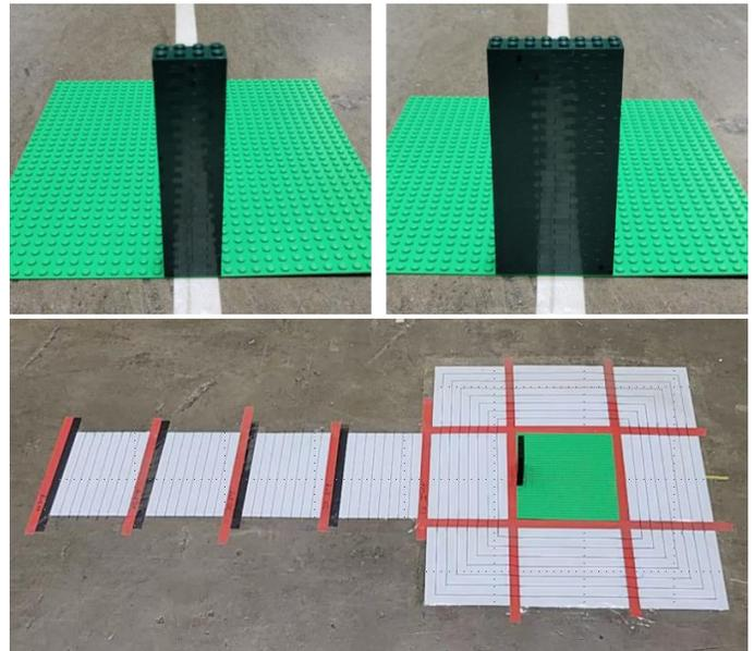
**FIGURE 8:** THE SMALL OBSTACLES WITH BASES (TOP), AND A GRID INSTALLED (BOTTOM)
