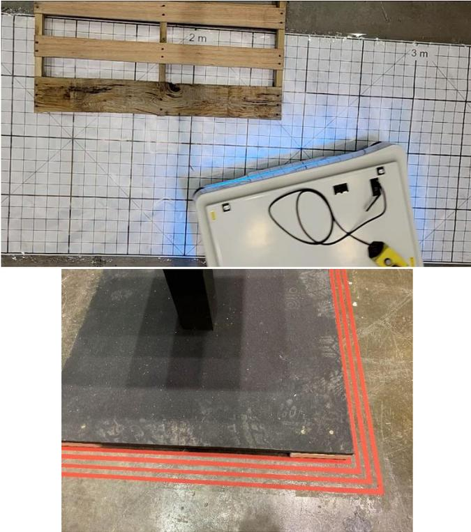
**FIGURE 6:** A PALLET ON A PRINTED PAPER GRID (TOP) AND THE TAPED GRID AROUND A WIDE BASE WITH CENTER POLE (BOTTOM)
