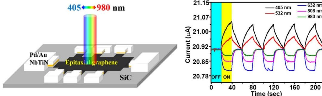
**Fig. 2.** (left) Schematic illustration of the EG/4H-SiC-based device and two-probe photodetector measurement setup with IBL under EG. (right) Dynamic photoresponse of the EG/4H-SiC-based device under 405 nm, 532 nm, 632 nm, 808 nm, and 980 nm excitation of intensity  $79.6\text{ mW/cm}^2$  at  $V_{DS} = 1\text{ V}$ . The switching behaviour of the device is marked as ON, and OFF in the first cycle.
