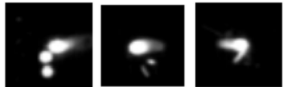
FIGURE 6: EXAMPLES OF ANOMALOUS, MELT-POOL IMAGES
