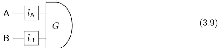
If the loss channel parameters  $l_A$  and  $l_B$  satisfy  $l_A + l_B \geq 1$ , then this effective Gaussian measurement is separable.
