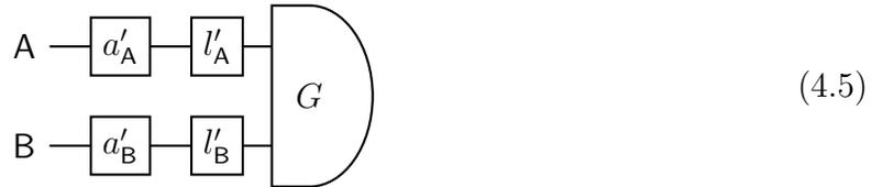
for loss parameters  $l'_A = l_A + n_A$  and  $l'_B = l_B + n_B$  and amplification parameters  $a'_A$  and  $a'_B$ . Applying Prop. 4.1 immediately gives the condition for separability  $l_A + l_B + n_A + n_B \geq 1$ .  $\square$
