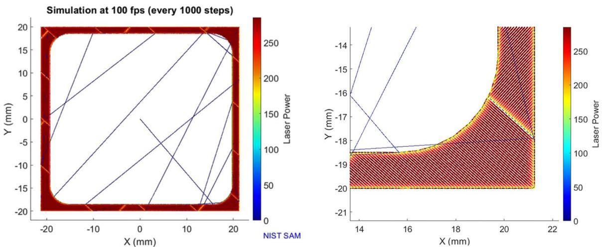
Fig. 11 Simulation of the generated process plans (left) at 100 frames per second (fps) with the “exact\_stop” mode and the “constant\_power\_mode”, the simulated scan paths (right), and the laser power gradient
