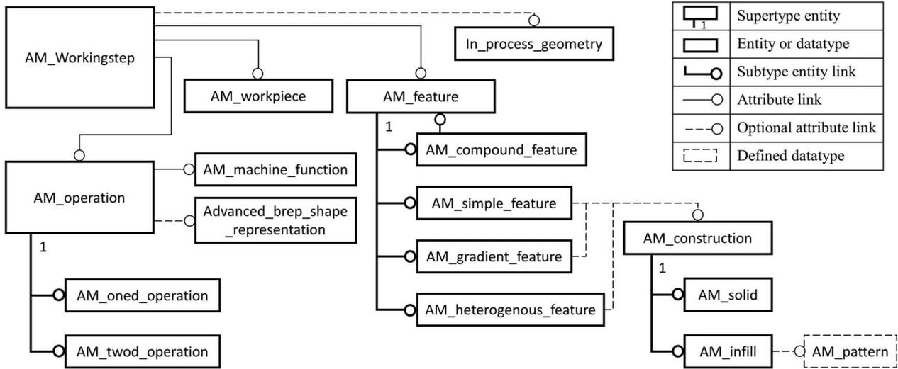
Fig. 2 A diagram representation of the ISO 14649-17 (part-17) standard entities applicable for PBF
