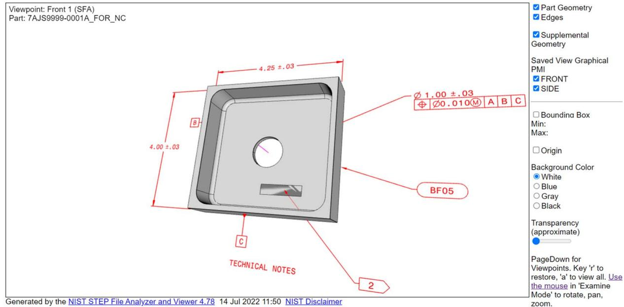
Fig. 8 A 3D model of the test part as shown in the NIST STEP File Analyzer and Viewer [39]
