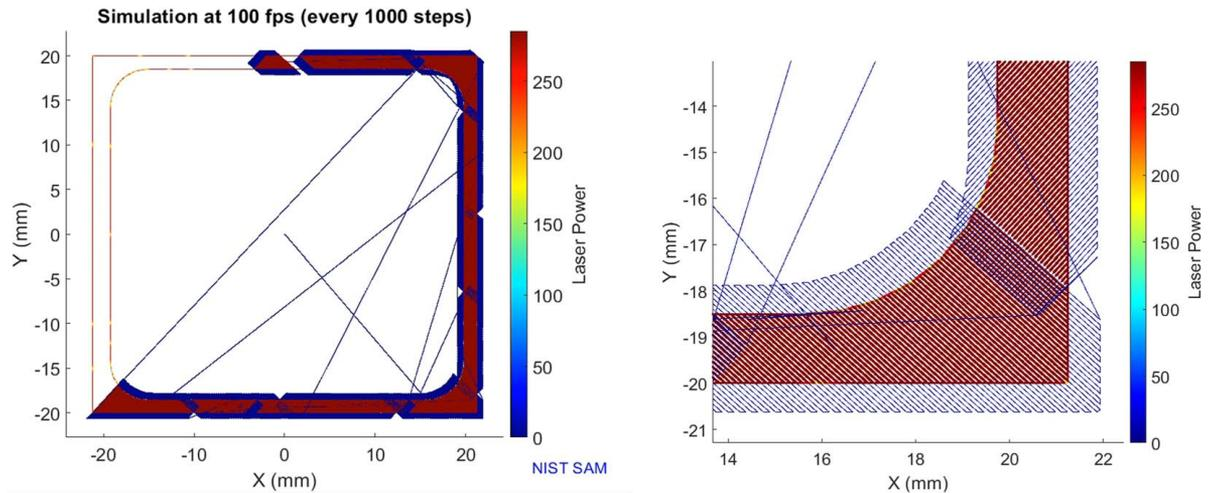
Fig. 10 Simulation of the generated process plans (left) at 100 frames per second (fps) using the “constant\_build\_speed” mode and the “constant\_power\_mode”, and a closer look at the simulated scan paths (right), along with the laser power gradient
