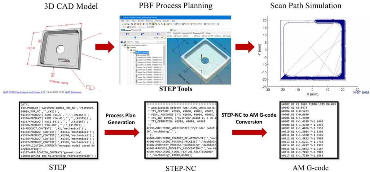
Fig. 9 Steps for PBF process plan generation and scan path simulation, and the data files shown below each step
