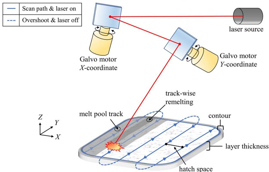
**Fig. 4** An illustration of the optical scan controller and process parameters for LPBF
