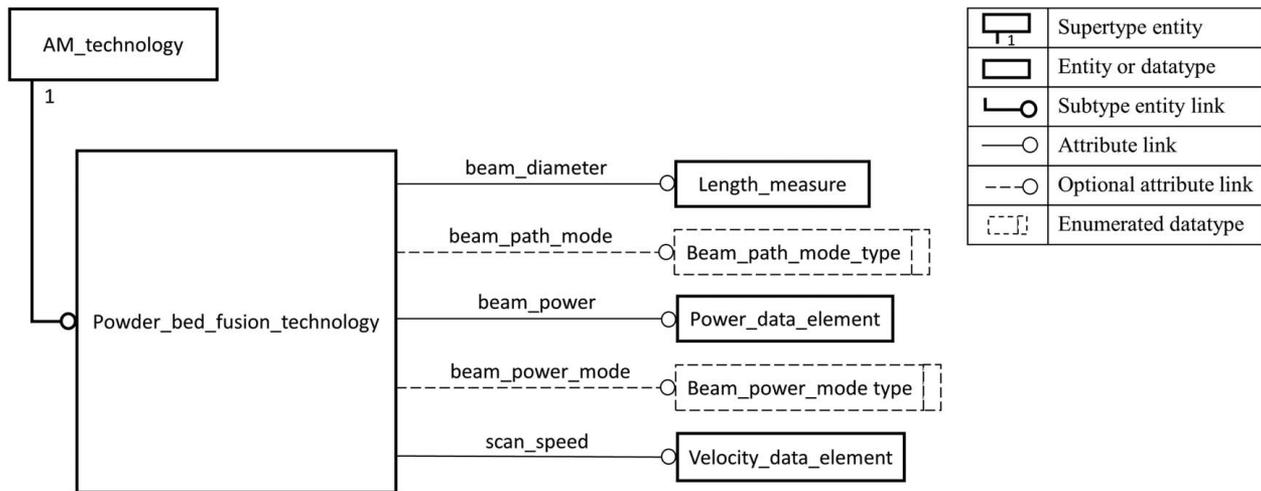
Fig. 7 A diagram of the “Powder\_bed\_fusion\_technology” entity
