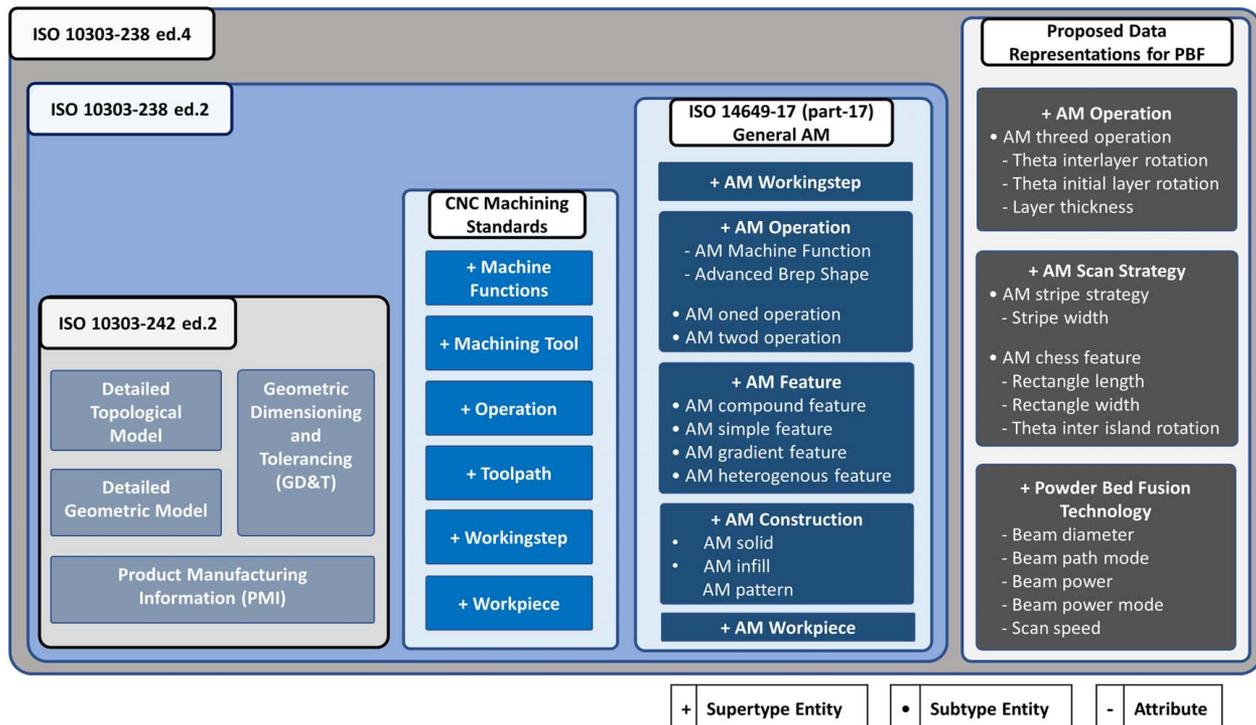
Fig. 1 A diagram that highlights the relationship between the STEP and STEP-NC standards and data representations
