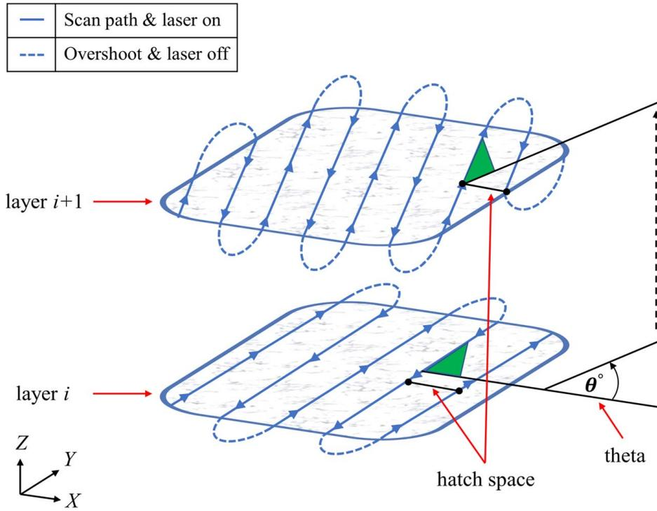
Fig. 5 An illustration of the “theta interlayer rotation” of a scan strategy between the layers  $i$  and  $i + 1$ , respectively, with the same hatch space
