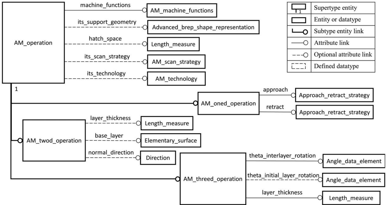
**Fig. 3** A diagram representation of the amended “AM\_operation” entity and the proposed “AM\_threed\_operation” entity
