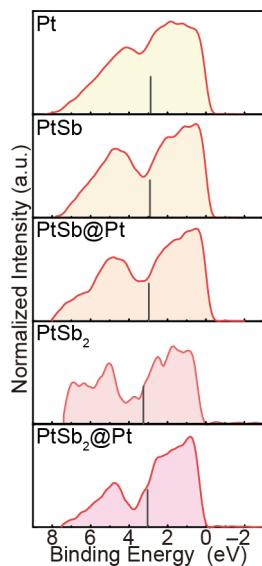
**Figure 4.** (a) X-ray photoelectron spectroscopy (XPS) valence band spectra. The gray vertical lines designate the valence band center ( $\epsilon_d$ ). The Fermi level is at 0 eV.
