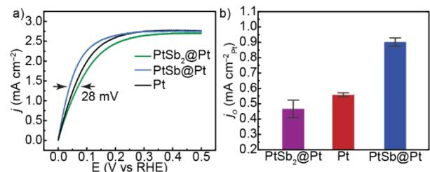
**Figure 3.** Hydrogen oxidation performance of Pt, PtSb<sub>2</sub>@Pt, and PtSb@Pt measured by (a) linear sweep voltammetry normalized by the geometrical area on a rotating-disk electrode at 1600 rpm and a sweep rate of 5 mV s<sup>-1</sup>, and (b) the mass-transport-corrected exchange current density ( $j_{\text{o}}$ ) normalized by the electrochemically active surface area on a Pt basis.
