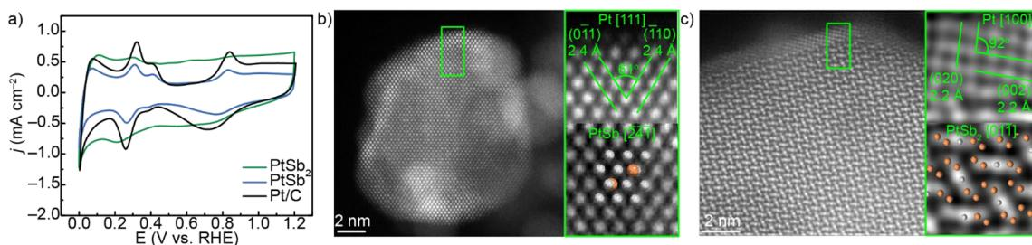
**Figure 2.** (a) Stabilized cyclic voltammograms (CVs) normalized by the geometric area. (b) STEM/HRTEM image for PtSb nanoparticles after cycling, showing that a PtSb@Pt structure has formed. (c) STEM/HRTEM image for PtSb<sub>2</sub> nanoparticles after cycling, showing that a PtSb<sub>2</sub>@Pt structure has formed.
