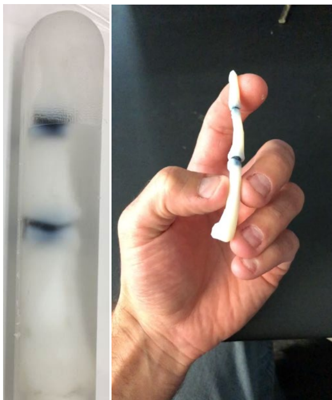
Figure 3 - Fingerprint target cast in clear PDMS material (left) with flexible 3D-printed bone (right) embedded
