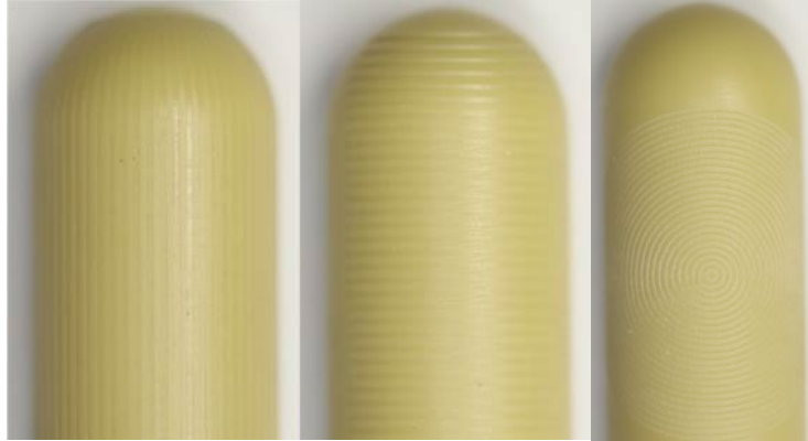
Figure 1 - Geometric target patterns engraved in rigid polycarbonate material: Vertical Ronchi (left), horizontal Ronchi (center), and concentric circular (right)
