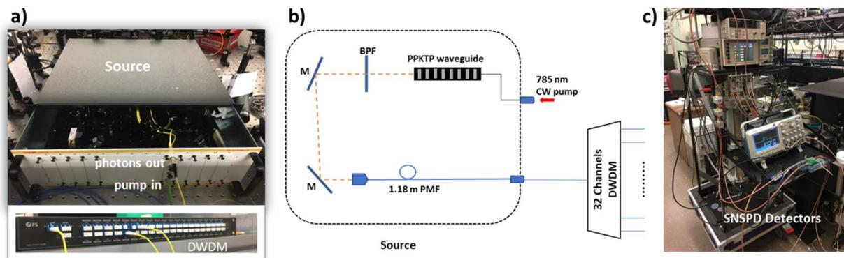
Figure 1: Portable Entangled Photon Source and SNSPD detectors for quantum network applications, **a)** photo of the portable source and DWDM, **b)** schematic of the Portable Entangled Photon Source connected to DWDM; M: Mirror, PMF: Polarization-Maintaining Fiber, BPF: Band Pass F, **c)** photo of the portable SNSPD detectors.
