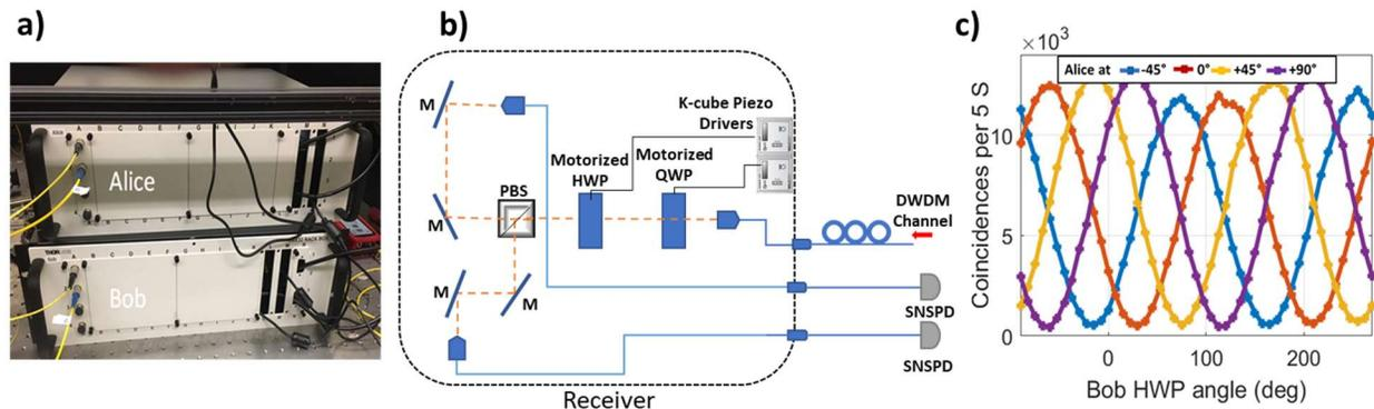
Figure 2: Portable polarization-entanglement analyzers (receivers), **a**) photo of two receivers boxes, Alice and Bob **b**) Setup schematic of the receiver, QWP: quarter-wave plate, HWP: half-wave plate; PBS: polarizing beam splitter. **c**) Polarization entanglement fringes as measured in different bases.
