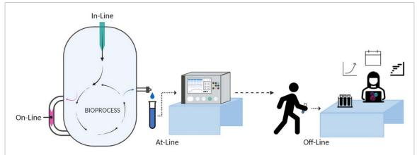
Figure 4. Diagram illustrating in-line, on-line, at-line, and off-line measurements in a TEMP bioprocess (graphic created with BioRender.com).
