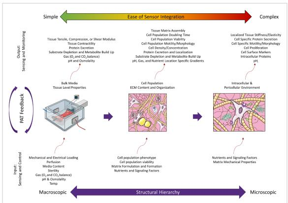
**Figure 5.** Sensing of an attribute is a data snapshot within a complex dynamic multi-scale system. Sensing is required as both an input and output of the system and can be representative of an attribute across different structural scales. The difficulty of conducting a measurement increases as the environment that is being sensed gets smaller and the measurement more specialized. Any attribute measurement must be contextualized within the full spectrum of the tissue culture system.
