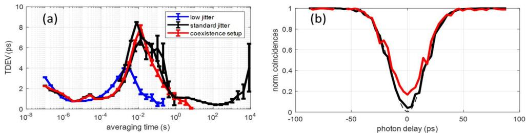
Figure 2. (a) White Rabbit TDEV vs. averaging time for the low-jitter (blue), the standard-jitter system (black) and the integrated coexistence setup (black), respectively. (b) simulated HOM interference for the standard White Rabbit system with/without background noise (red/black line) and without jitter or noise (black dashed line)
