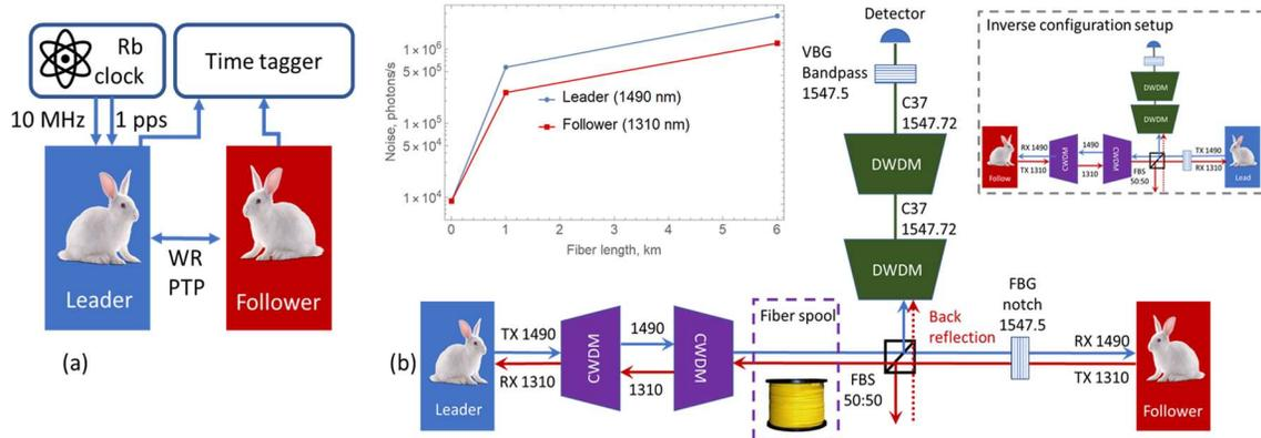
Figure 1. (a) White Rabbit leader-follower scheme. (b) Noise measurements setup and results in a quantum channel at 1547.5 nm, coexisting with the WR synchronization signals at 1310 nm and 1490 nm in the same fiber. Right Inset: The same setup, reversed. Left Inset: Background photons vs fiber length. Measured number of photons is adjusted for nominal loss in optical components.
