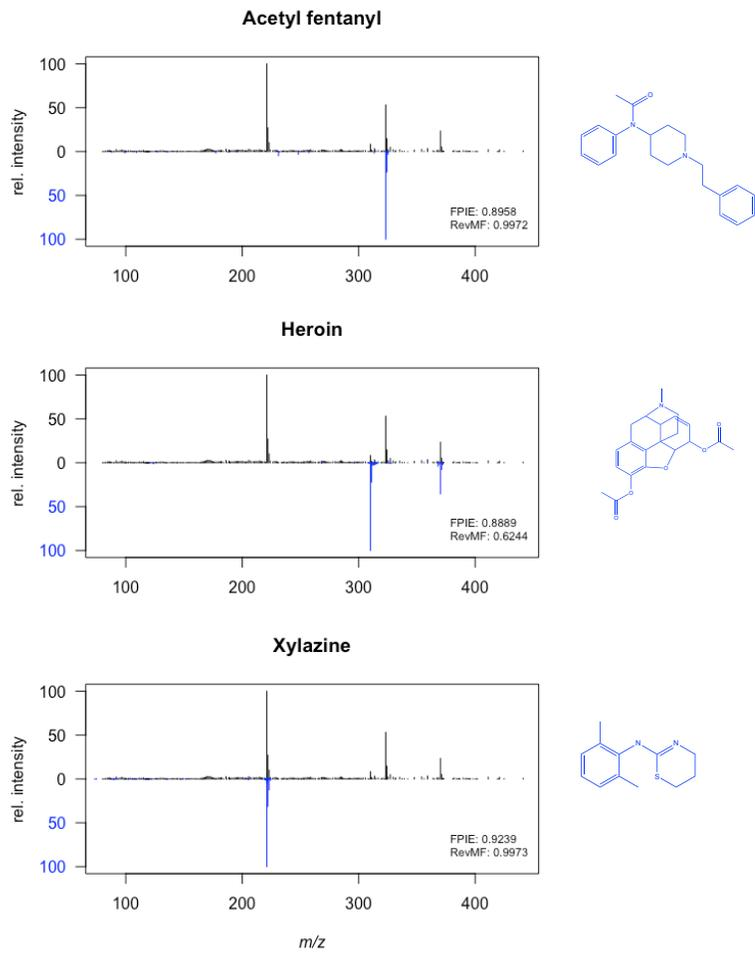
Figure 3: Head-to-tail comparisons of query in-source collision induced dissociation mass spectra collected at +30V (black/top) with library spectra of acetyl fentanyl, heroin and xylazine collected at +30V (bottom/blue). Molecular structures of each library compound included for reference.
