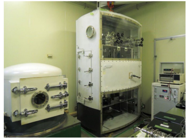
Figure 25. The balances of the static gravimetric system of NMIJ/AIST.
