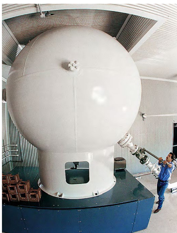
Figure 23. A gravimetric standard for flows up to 43 \text{ kg s}^{-1} ( 2000 \text{ m}^3 \text{ min}^{-1} ) at the Southwest Research Institute. Reproduced with permission from [74]. Photo courtesy of Southwest Research Institute.
