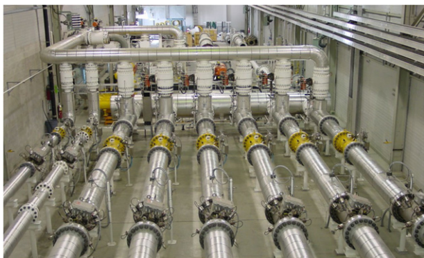
Figure 45. Multipath ultrasonic time-of-flight meters at Trans Canada Calibrations are used in parallel to perform natural gas flow calibrations up to 12 \text{ kg s}^{-1} ( 917 \text{ m}^3 \text{ min}^{-1} ). Photo courtesy of TransCanada Calibrations Ltd.
