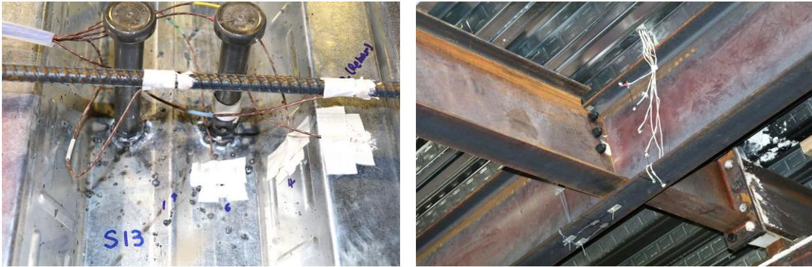
**Fig. 53. Photographs of typical thermocouples installed in the composite girder near its midspan.**
