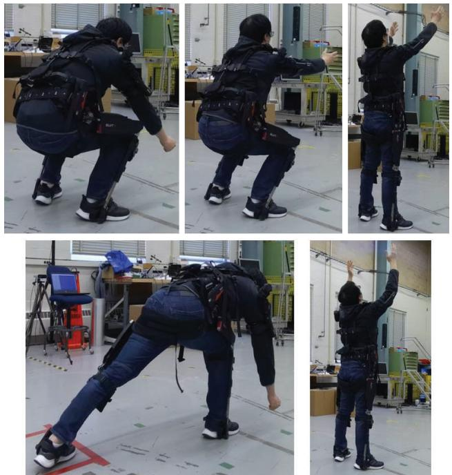
Figure 2. Load alignment poses (Top) and applied force poses (Bottom) cameras were triggered using the manufacturer-provided synchronization system. The OTS was calibrated per manufacturer's documentation on a weekly basis using a calibration bar. Figure 3 illustrates the experimental setup.
