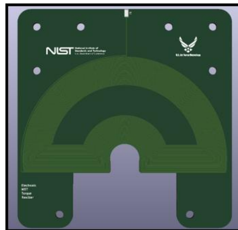
Figure 3. CAD model of the top side of a single 0.8 mm thick PCB. A total of 33 turns are printed on each side. At the top of the PCB are two bare solder pads, allowing for stacking and soldering in series. A stack of 8 PCBs with 528 turns has a total resistance of about 120 \Omega .
