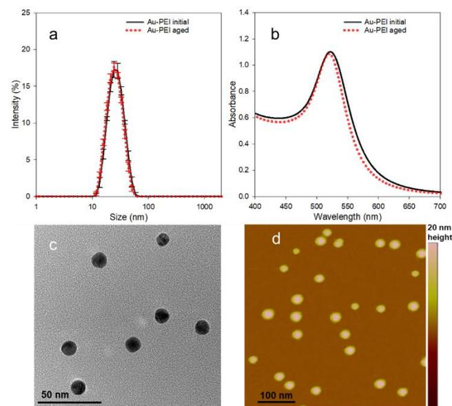
Fig. 1. Representative measurements data of Au-PEI@NIST; (a) intensity-weighted size distribution by DLS, (b) SPR band by UV-Vis, (c) TEM image (Scale bar is 50 nm), and (d) AFM image (Z-scale for height is 20 nm and scale bar for width is 100 nm; *Note:* The apparent width of the particles are larger than their height due to the intrinsic tip convolution effects in AFM imaging).
