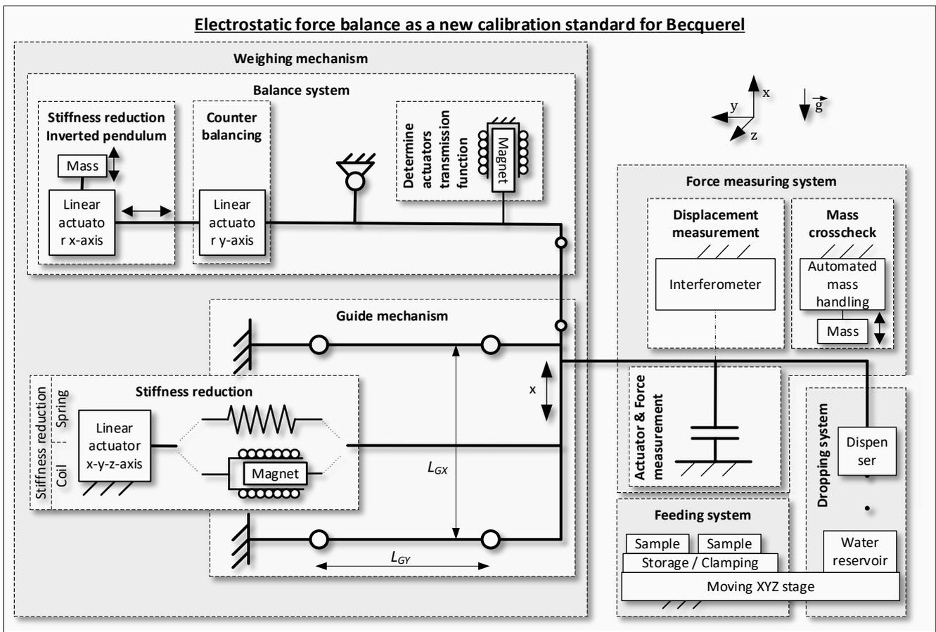
Figure 2. Technical principle of the electrostatic force
