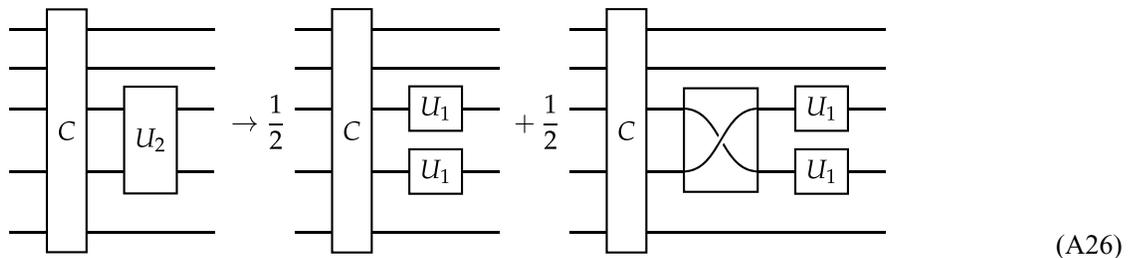
*b. Type B* The gate of type B has a noiseless two-qubit gate followed by dephasing on one of the outgoing legs. The dephasing is also followed by a single-qubit random gate. To simplify things, we first understand the effect of the channel
