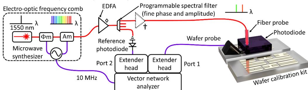
Fig. 1. Schematic diagram of the millimeter-wave source with phase and amplitude control. An electro-optic frequency comb is amplified by an EDFA and filtered by a programmable spectral filter. Two or more comb lines are filtered and phase- and amplitude-shifted to generate single- or multi-tone programmable waveforms. On-wafer measurement with a vector network analyzer lets us characterize the system performance at the edge of the photodiode chip.
