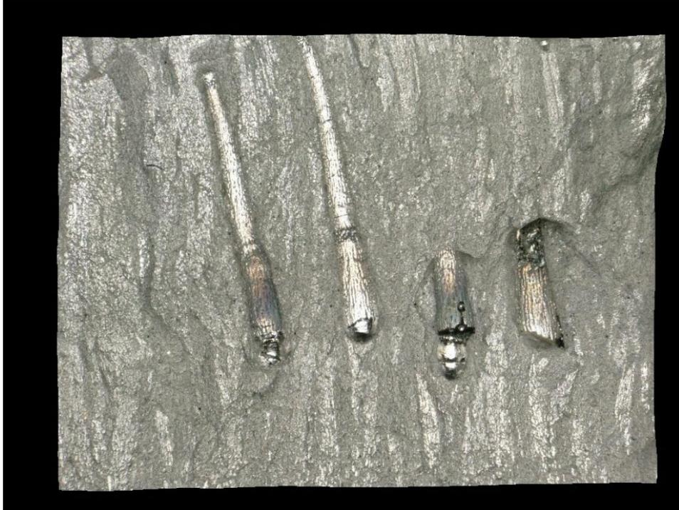
Specimen W1-C4, left side: detail of the wormhole cavities
