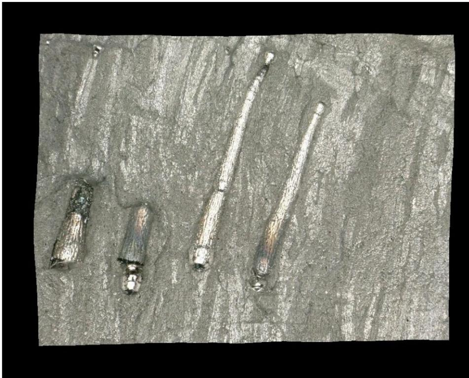
Specimen W1-C4, right side: detail of the wormhole cavities
