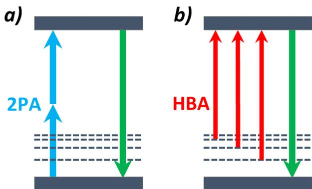
**Figure 1.** Schematic of 2PA (a) and HBA (b) with electronic and vibronic levels indicated by solid and dashed lines, respectively. The 2PA excitation source (blue) may have high-energy components (red) that resonate with 1PA (hot-band) transitions. Note that the fluorescence emitted by the two mechanisms (green arrows) is indistinguishable.
