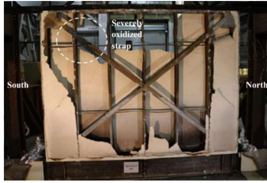
Figure 5. Photograph of the fire exposed side of the wall in Test S02 after the fire test (before cycling) [1].
