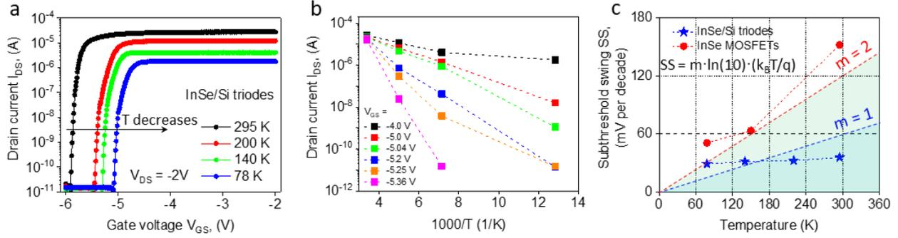
**Figure 4. Temperature-dependent electrical characteristics of InSe/Si 2D/3D triodes.** (a) Temperature-dependent  $I_{DS}$ - $V_{GS}$  transfer characteristics measured at  $V_{DS} = -2.0$  V. (b) Arrhenius plot of drain current as a function of  $1000/T$  for various gate voltages. (c) Subthreshold swing as a function of temperature for InSe/Si 2D/3D heterojunction tunneling triodes and InSe control MOSFETs.
