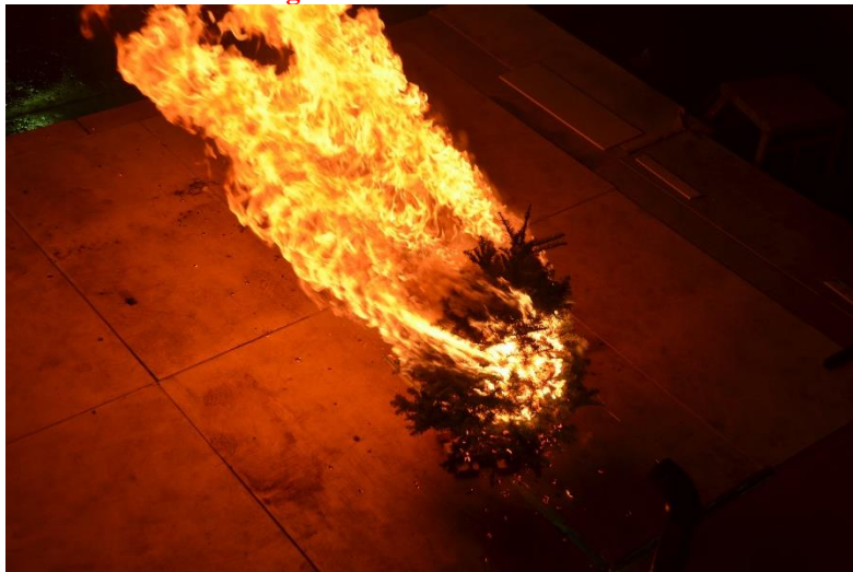
Ensuing combustion from firebrand ignition
