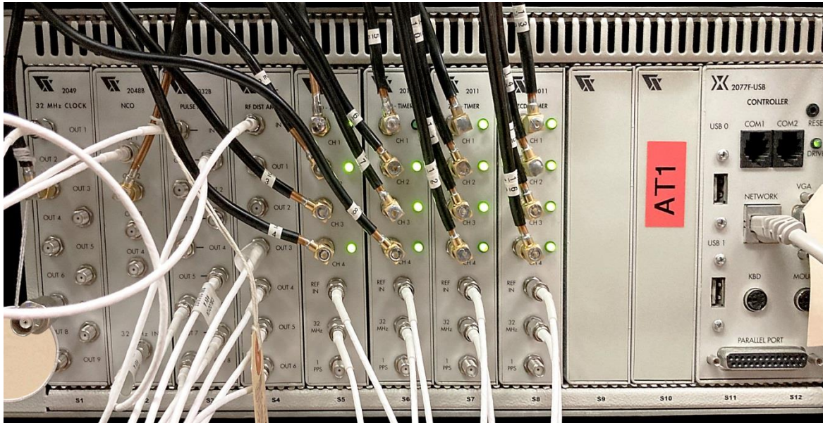
Fig. I.A.8. Photograph of a MCMS chassis with 16 clock measurement channels. Modules from right to left: industrial embedded computer, four measurement modules implementing DMTD, distribution amplifiers and sources for the 32 MHz onboard quartz oscillator counting time base and NCO synthesizer signals.
