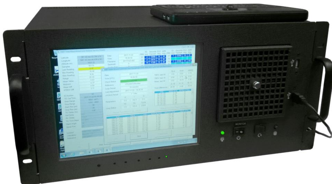
Fig. II.C.4. NIST's implementation of the MSCVDC, the NIST disciplined clock (NISTDC).
