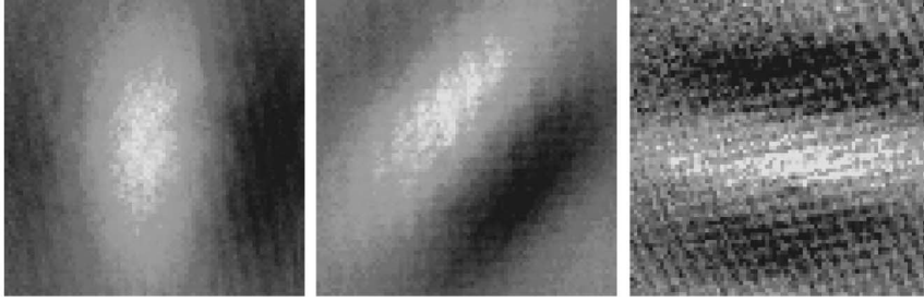
Fig. 1. – Interference fringe data generated by a simulated rotation. The atom fringe orientation measures the system rotation direction; the fringe period measures the system rotation magnitude. Left: \Omega_y = 35 mrad/s. Center: \Omega_x = \Omega_y = 25 mrad/s. Right: \Omega_x = 89 mrad/s.
