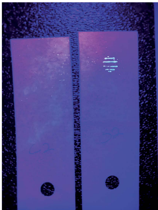
Fig. 3 Fluorescent optical image of two CN wipes after manual wiping a vinyl surface containing 20 \mu\text{m} PLS microspheres. The unmodified wipe (left) was first manually swiped over the surface of a vinyl sample containing dry deposited fluorescent PSLs. The score wipe (right) was then translated over the same location on the microsphere-containing vinyl surface without the addition of any additional PSL microspheres. The scores were produced with the razor cutting system to coincide with the limited circular area of the wipe interrogated by the thermal desorber of a typical APF system. The width of the CN wipe is 2.54 cm.
