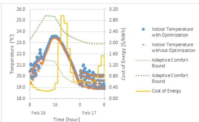
**FIGURE 8: INDOOR TEMPERATURE IN FEBRUARY DURING A TIME OF HIGH PRICE INCREASE**
