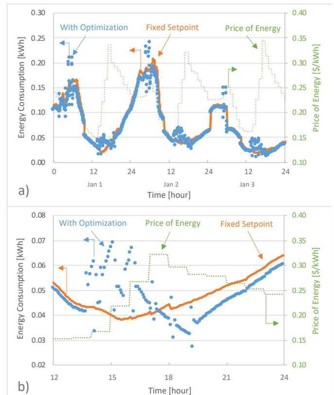
**FIGURE 6a:** ENERGY CONSUMPTION FOR THE TWO CASES OVER THE THREE-DAY TIME PERIOD WITH THE PRICE OF ENERGY AT EACH TIMESTEP
