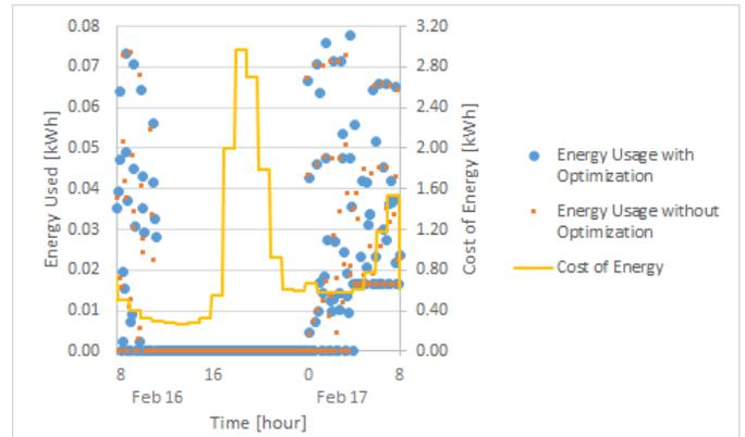
**FIGURE 9: ENERGY CONSUMPTION IN FEBRUARY DURING A TIME OF HIGH PRICE INCREASE**
