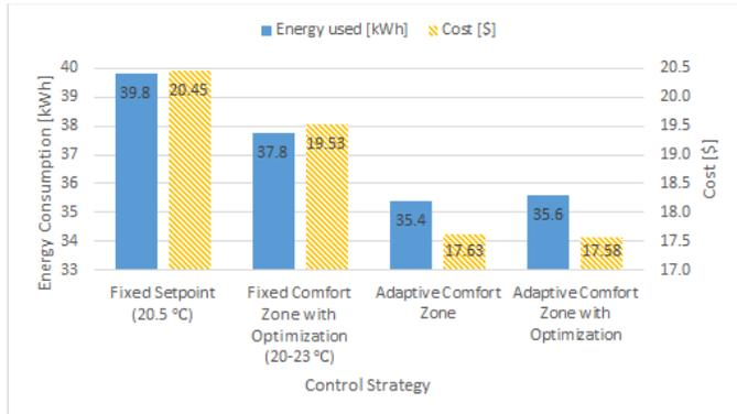
**FIGURE 4:** ENERGY CONSUMPTION AND COST FOR EACH HVAC CONTROL STRATEGY FOR FEBRUARY 12-18
