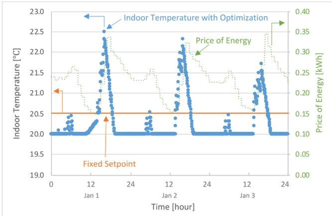
**FIGURE 7: INDOOR TEMPERATURE FOR THE TWO CASES OVER THE THREE-DAY TIME PERIOD WITH THE PRICE OF ENERGY AT EACH TIMESTEP**
