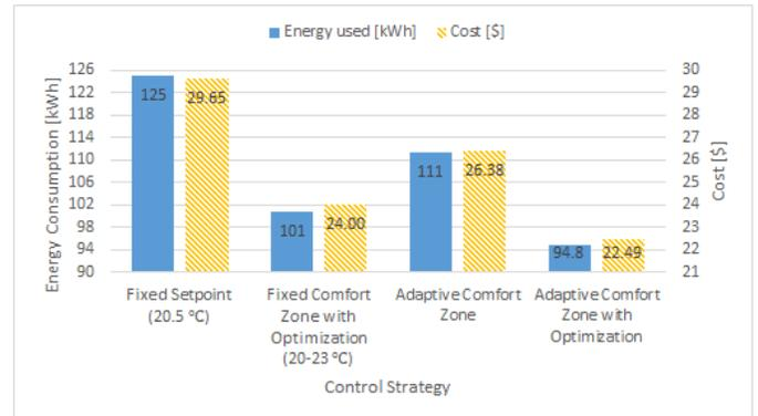
**FIGURE 3:** ENERGY CONSUMPTION AND COST FOR EACH HVAC CONTROL STRATEGY FOR JANUARY 1-7
