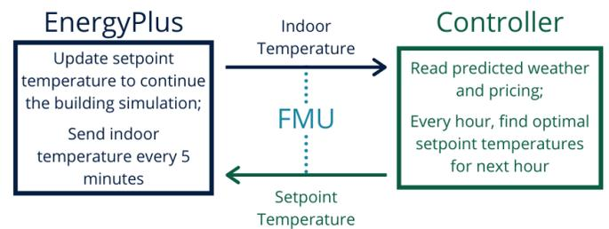
**FIGURE 1: THE EXCHANGE OF INFORMATION BETWEEN ENERGYPLUS AND THE CO-SIMULATION PLATFORM TO FIND THE OPTIMAL SETPOINT TEMPERATURE**
