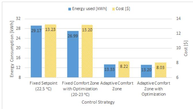
**FIGURE 5:** ENERGY CONSUMPTION AND COST FOR EACH HVAC CONTROL STRATEGY FOR SEPTEMBER 27 – OCTOBER 3
