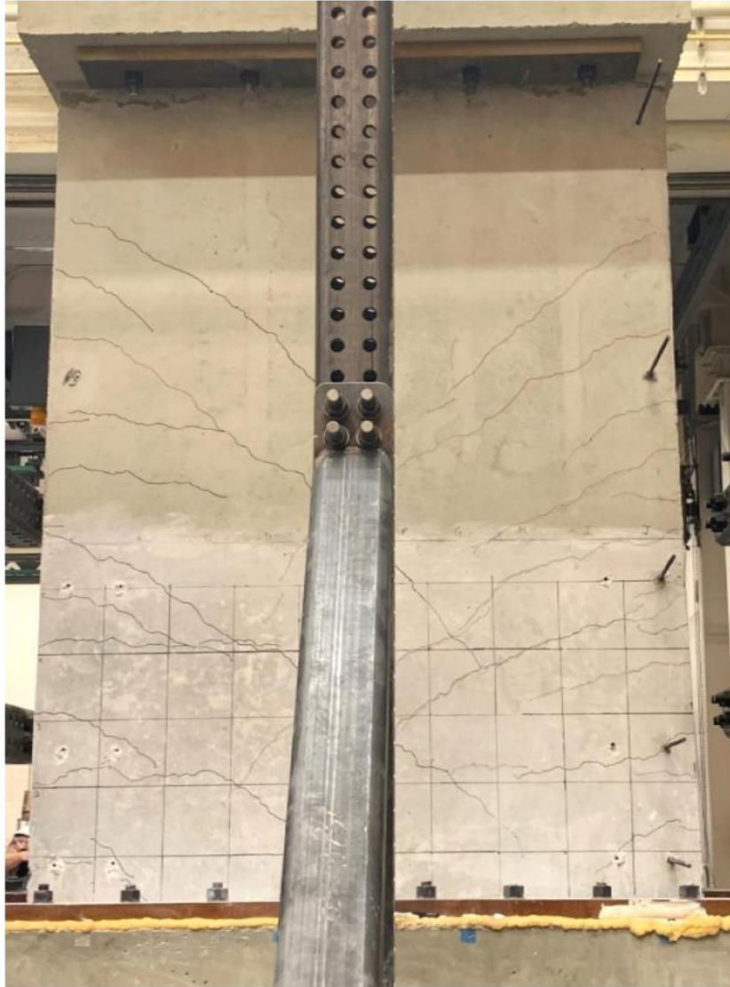
**Figure 3.4. Cracks on the west face of Wall 4 at a drift ratio of 1.000 % (Cycle 17). Cracks highlighted using permanent marker.**
