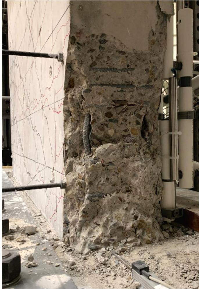
**Figure 3.7. Spalling of concrete in compression zone of Wall 4 at a drift ratio of 3.000 % (Cycle 29) exposing buckled reinforcement in the boundary element**
