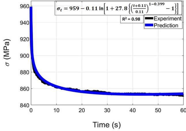
Figure 6:  $\sigma$  vs  $t$  predicted using equation (1)
