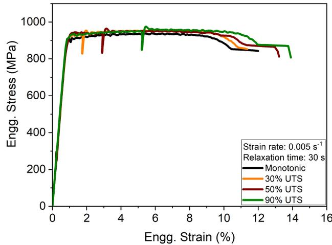
Figure 2: Stress-strain curve for sample subjected to stress relaxation at various pre-strain for 30 s hold time
