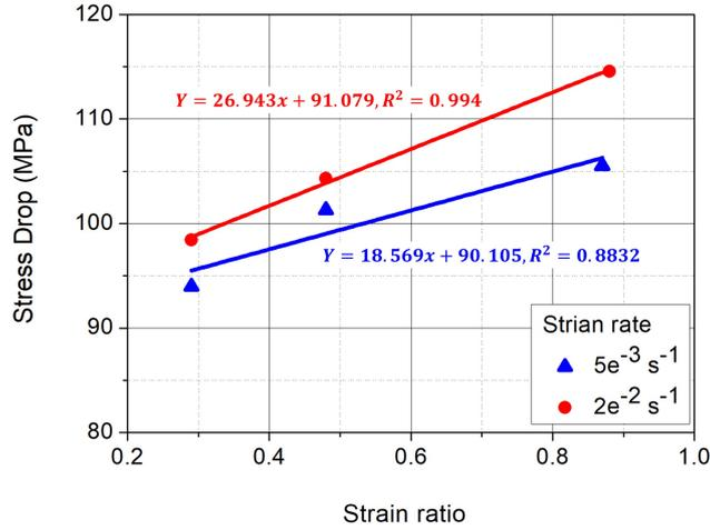
Figure 5: Stress drop during relaxation in Ti-6Al-4V alloy (Relaxation time = 30 s)
