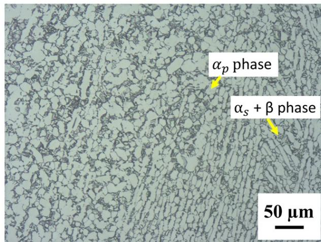
Figure 1: Microstructure of as received Ti-6Al-4V alloy
