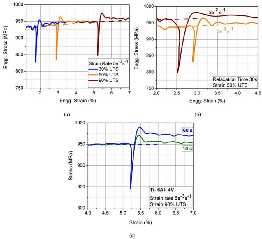
Figure 4: Stress jump post relaxation showing the effect of (a) Pre-strain, (b) Strain rate, (c) Relaxation time
