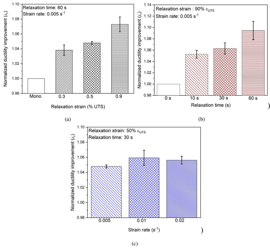
Figure 3: Ductility improvement due to stress relaxation showing the effect of (a) Pre-strain, (b) Relaxation time (c) Strain rate
