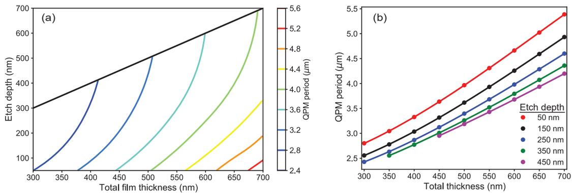
Fig. 2. (a) Required QPM periods as a function of LN film thickness and etch depth with waveguide width set to 1200 nm. The top left portion of the plot above the solid black line represent unphysical structures. (b) Dependence of QPM period on total LN film thickness (1200 nm waveguide top width) for different etch depths. We observe a decrease in slope with larger etch depths.
