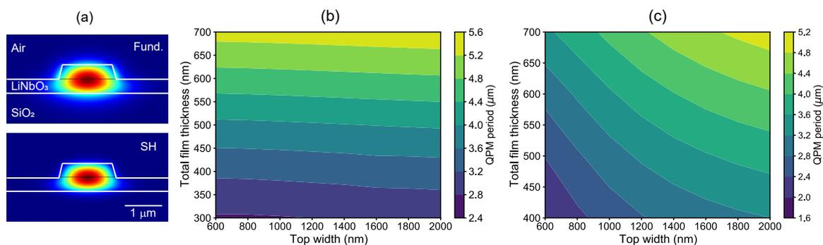
Fig. 1. (a) Calculated fundamental and second-harmonic TE modes. Required QPM period for different waveguide widths and thicknesses where etch depth is fixed to (b) 50 nm and (c) 350 nm.
