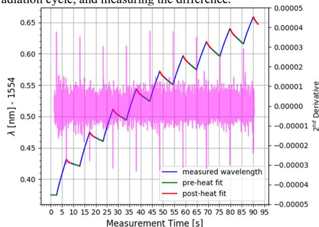
Fig 2. Resonance wavelength ( $\lambda$ ) of photonic calorimeter sensor during irradiation cycles. Differential heating was determined by extrapolating pre-heating (green) and post-heating (red) data to midpoints, determined by 2<sup>nd</sup> derivative (pink).
