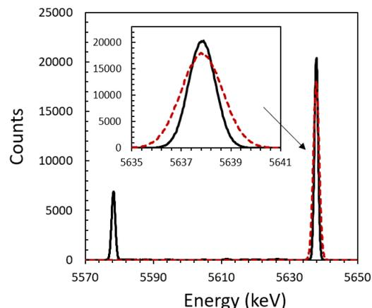
Fig. 1. Geant4 Monte Carlo simulation of Am-241 DES spectra for Au absorber of thickness 15  $\mu\text{m}$  (solid black) or 1000  $\mu\text{m}$  (dotted red). In the latter case, the  $\gamma$ -ray escape peak is absent and the activity is equal to the count rate in the peak located at the Q-value (right
