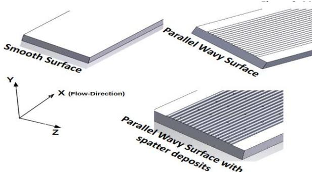
Figure 4. Modeled AM Surfaces
