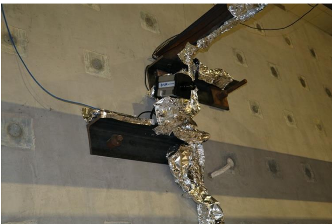
Fig. 3-8. Infrared camera mounted on the strong wall.
