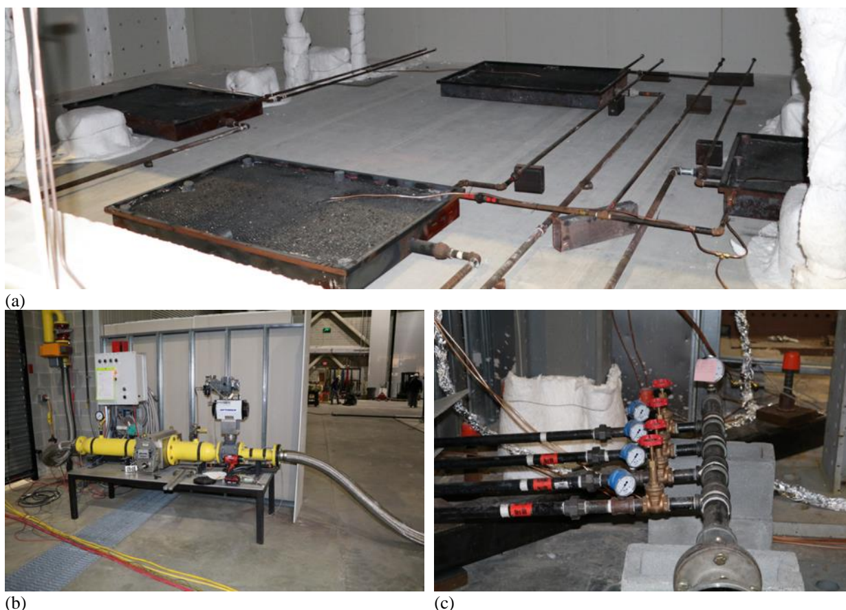
Fig. 2-36. Photographs of (a) burners placed inside of the fire test compartment, (b) NFRL's natural gas fuel delivery system; (c) balancing valves at upstream of the burners.
