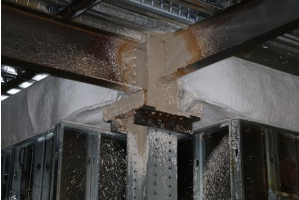
Fig. 2-35. Photographs of (a) enclosure around the beam-to-girder connection region; (b) enclosure around column (outside of the compartment).
