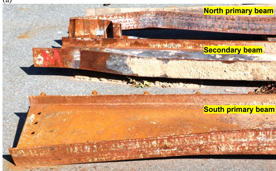
Fig. B-24. Post-test photographs of W16×31 beams in the test bay; (a) east end and (b) west end.
