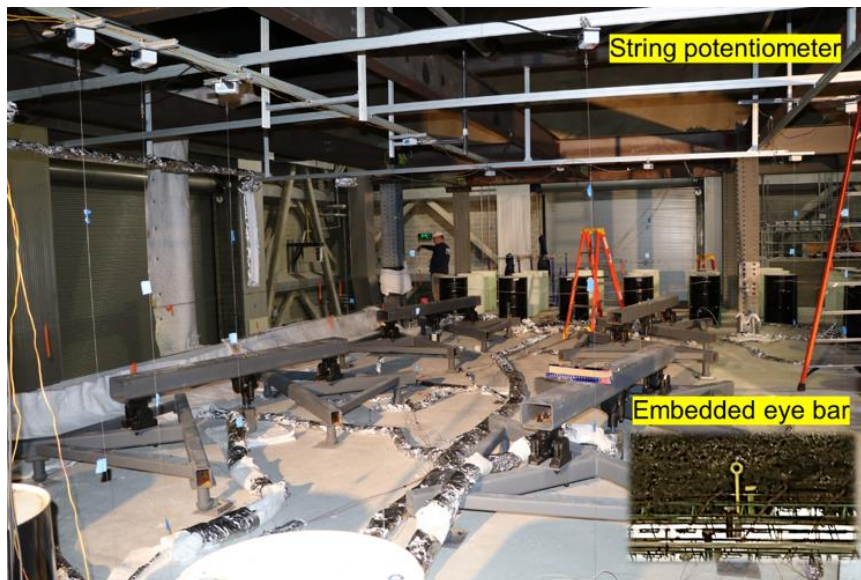
Fig. 3-2. String potentiometers used for the vertical displacement measurements. Measuring strings were directly attached to the eye bars partially embedded in the concrete slab.
