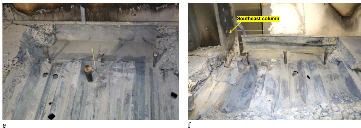
Fig. B-23. Post-test photographs of headed stud anchors in the test bay.
