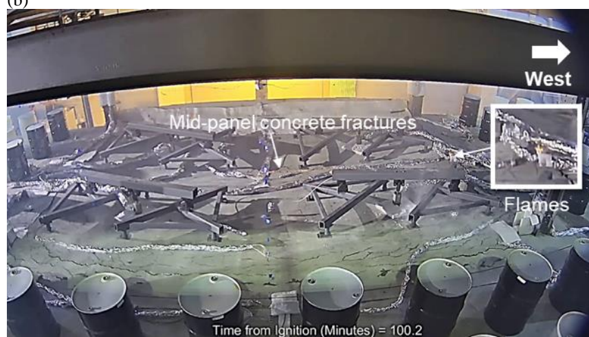
Fig. 4-27. Snapshots of the test video looking down on the top of the test floor assembly at about (a) 41 min, (b) 69 min, and (c) 100 min.
