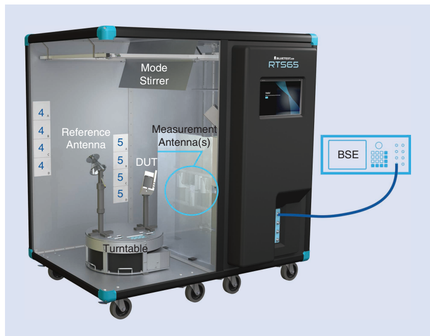
Figure 1. A reverberation-chamber setup for TIS, including a turntable for position stirring, which is needed in loaded chamber measurements. The DUT is connected to a BSE, and it is disconnected for the reference measurement of G_{ref} , where both the reference and measurement antenna are connected to a VNA.
