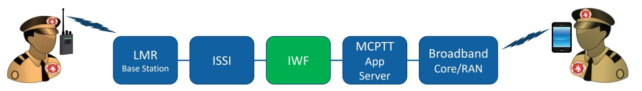
LMR-Land Mobile Radio MCPTT-Mission Critical Push-to-Talk MCData-Mission Critical Data ISSI-Inter RF Subsystem Interface
